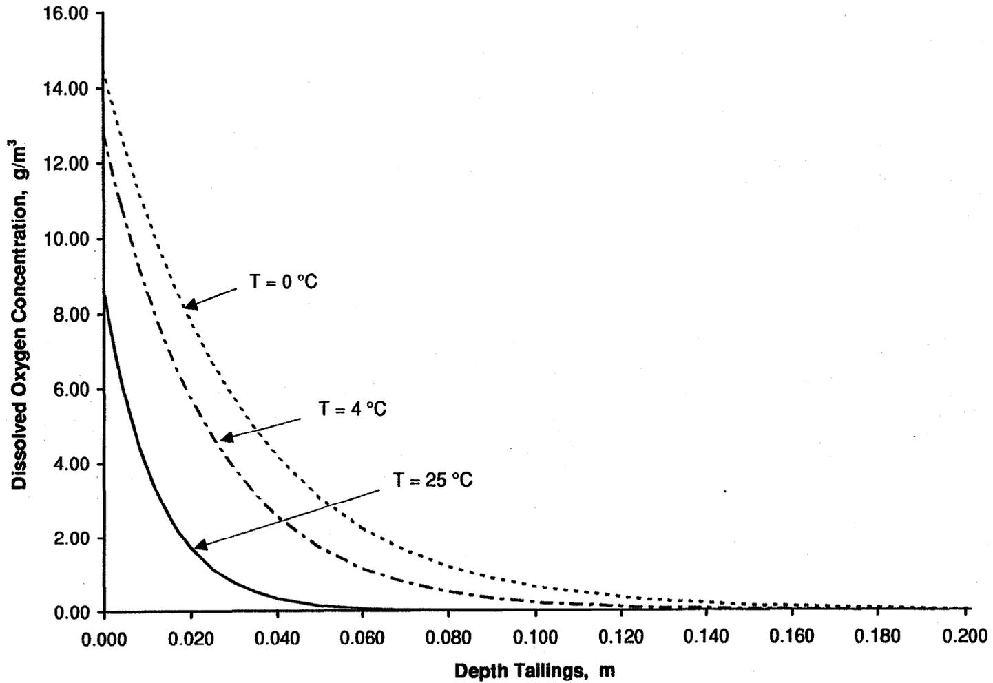
Figure 4.3 Dissolved oxygen concentration profiles (expanded scale) as a function of depth at 25°, 4°, and 0°C in saturated tailings (water filled pore spaces) with no additional cover. The air/tailings interface is at 0 m.
