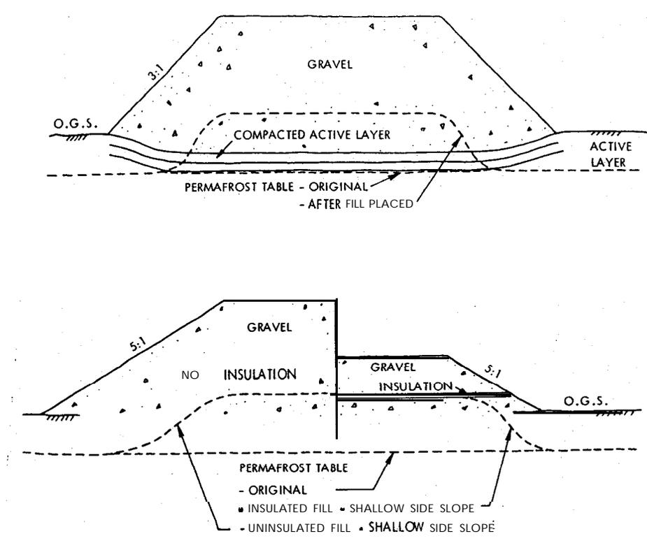
Figure 5.7 Impact of Insulated and Uninsulated Covers on Permafrost Table (after Johnston, 198 1)
