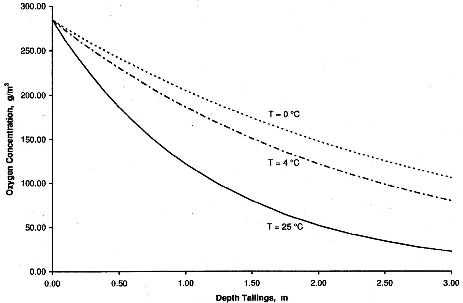
Figure 4.1 Oxygen concentration profiles as a function of depth at 25°, 4°, and 0°C in unsaturated tailings (air filled pore spaces) without cover. The air/tailings interface is at 0 m.
