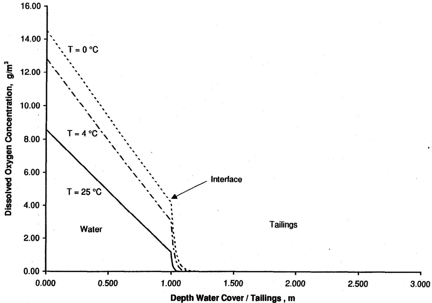
Figure 4.4 Dissolved oxygen concentration profiles as a function of depth at 25°, 4°, and 0°C in unmixed water cover of depth 1 m and underwater deposited tailings. The tailings-water interface is at depth 1.0 m from the surface of the water cover.
