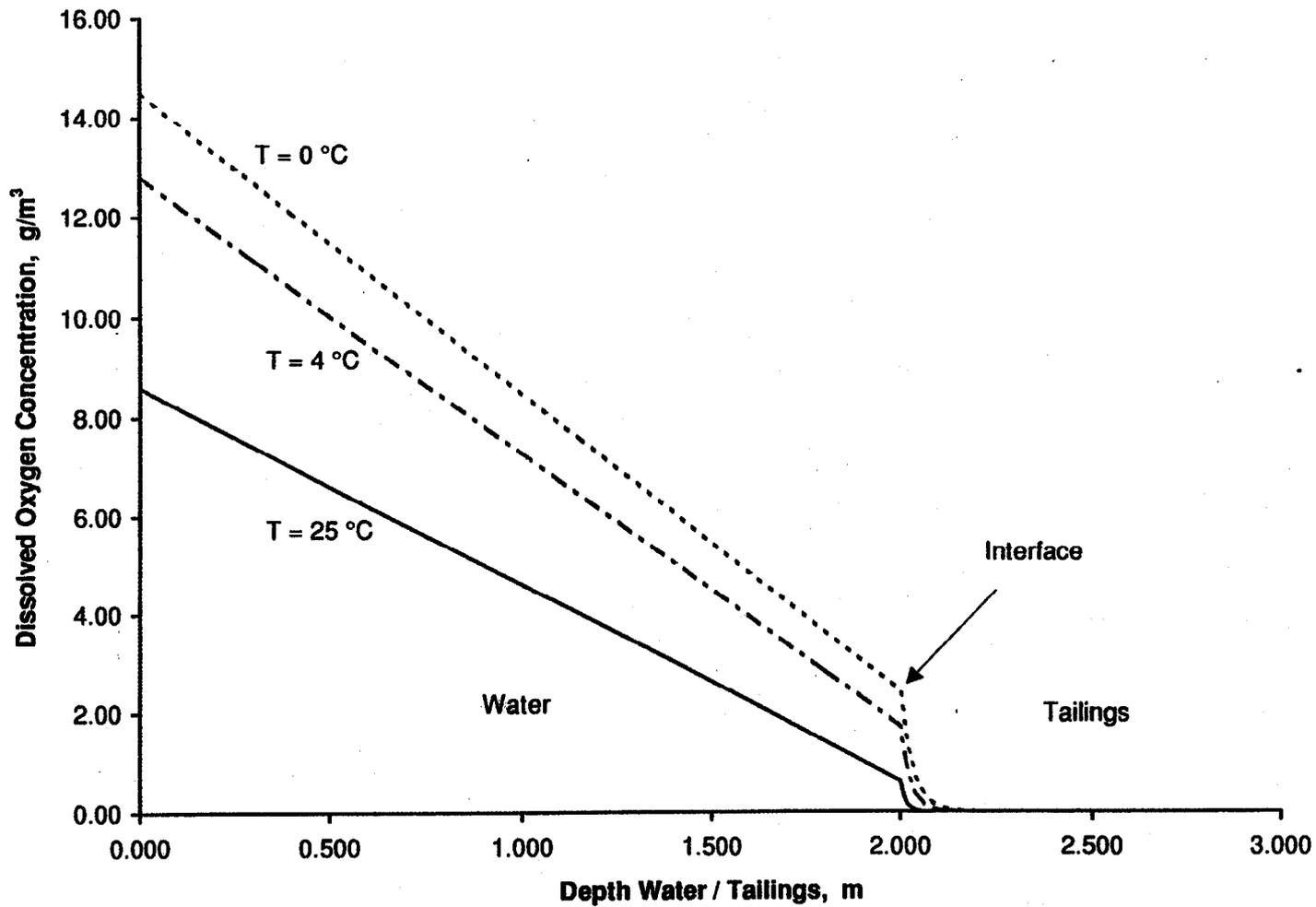
Figure 4.5 Dissolved oxygen concentration profiles as a function of depth at 25°, 4°, and 0°C in unmixed water cover of depth 2 m and underwater deposited tailings. The tailings-water interface is at depth 2.0 m from the surface of the water cover.
