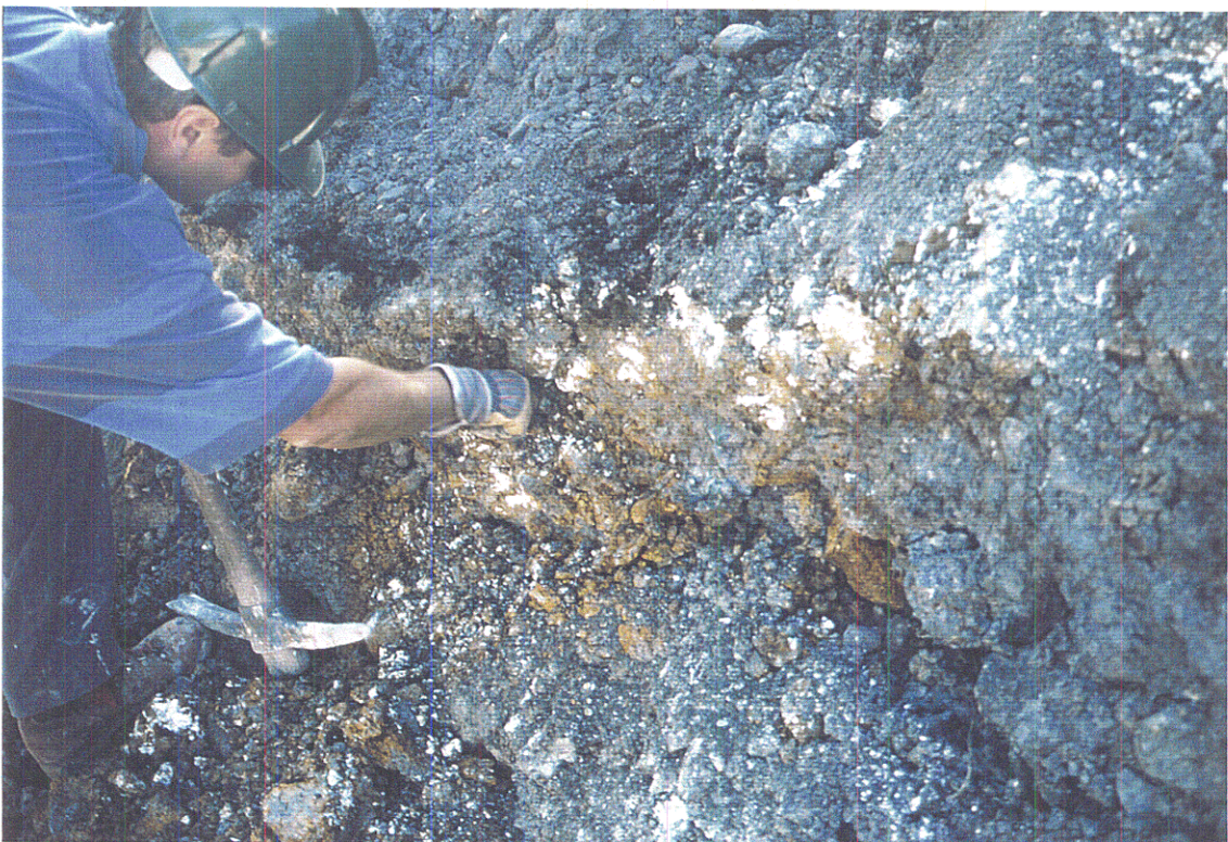
Photo 6. During dump disassembly; fresh-cut exposure of waste rock showing white paint confined above, and flowing over, an oxidized layer.
