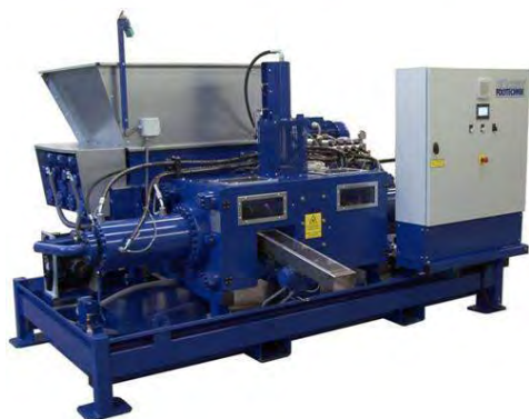
Figure 2 Höcker BrikStar press (left) was used for production of cylindrical briquettes with 5 cm in diameter (right)
