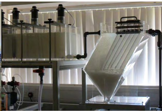
Figure 2. Close-up of the clarifier with subdued lighting showing ettringite precipitates and clear overflow
