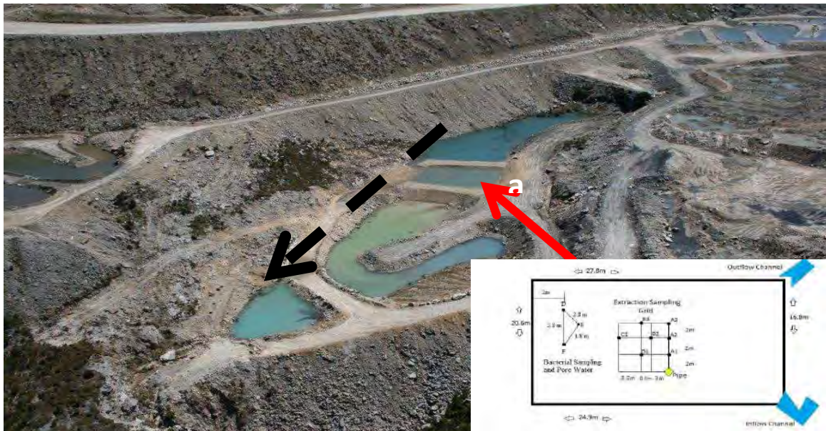
Figure 2 Emplacement of mussel shell bioreactor (location a); dashed line denotes direction of flow from the upper sediment pond, through the bioreactor and then two sediment ponds before discharge
