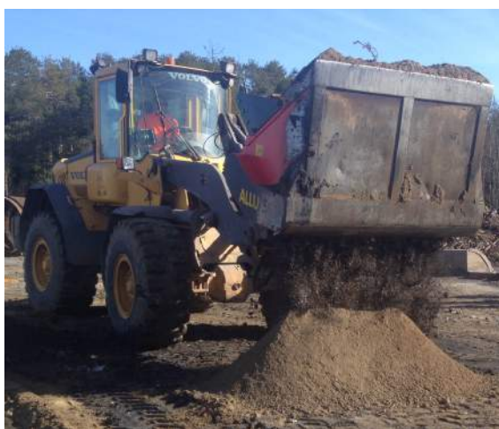
Figure 1 Loader with a crushing bucket
