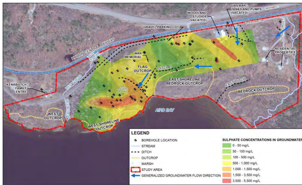
Figure 3 Sulfate concentrations in groundwater (mg/L)
