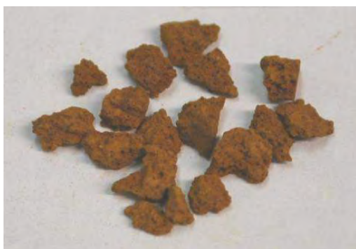
Figure 3 SHM-based adsorbents, obtained by mixing with an organic polymer (left) and high pressure compaction, crushing and sieving (right). Grain size: 1-2 mm in both pictures
