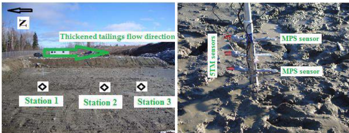
Figure 1 Experimental cell: a) Location of the different monitoring stations; b) details of instrumentation
