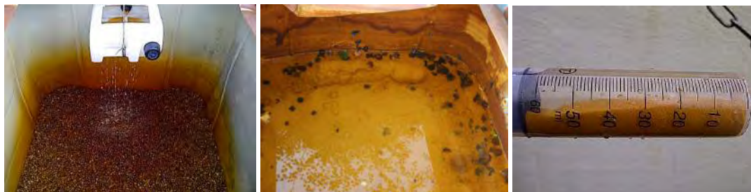
Figure 2 Left, initial stages of filling the VFR; centre: Ochre inside the VFR (after draining tank); right: ochre precipitates taken directly from the VFR.
