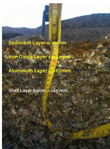
Figure 3 Geochemical gradient based on downward vertical flow within the mussel shell bioreactor
