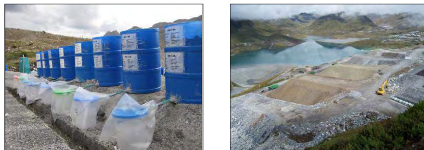
Figure 1 Experimental field barrels, 1m high and containing ~350 kg of waste rock (left); and experimental waste rock dumps, 10m high and containing ~30,000 kg of waste rock (right) at Antamina.
