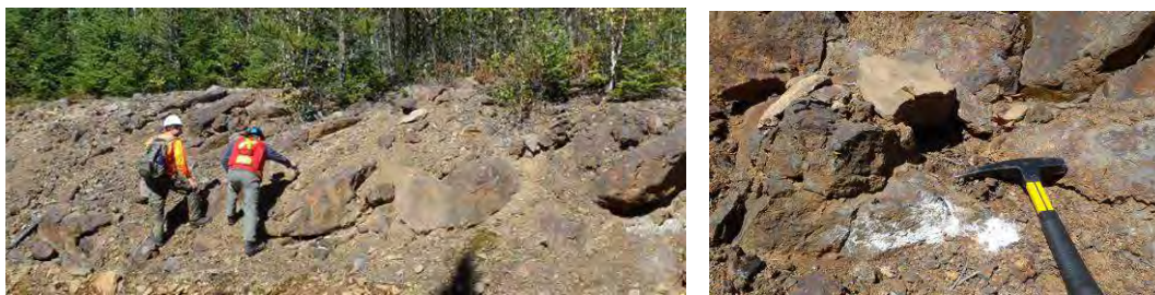
Figure 1 Left image shows example of a field sampling location where Duluth Complex rock was exposed during construction of a railroad. Right image shows “white crust” observed at the site.
