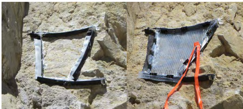
Photo 1 Typical Minewall station prior to leachate collection (left) and with cover between sampling events (right). Note that the upper horizontal structure of the Minewall measures ~50cm for scale.
