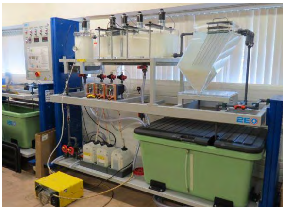
Figure 1. Photograph of plant in operation showing the ettringite precipitate in the clarifier and the external sludge recirculation pump in the foreground
