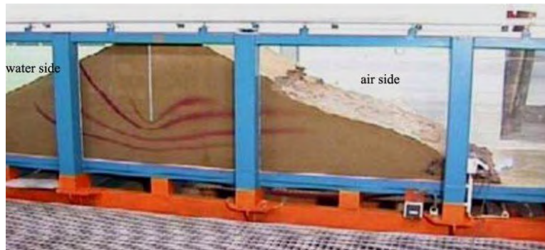
Figure 1 A physical model slope with slides on the air side (Aigner, 2004)
