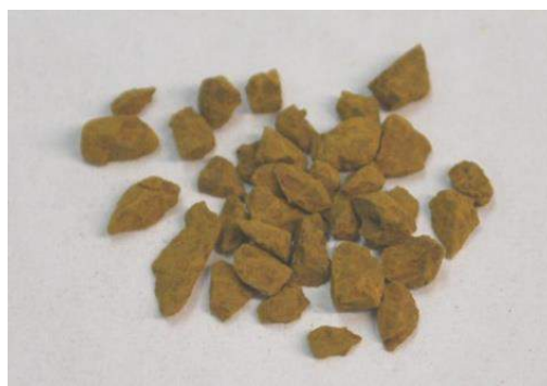
Figure 3 SHM-based adsorbents, obtained by mixing with an organic polymer (left) and high pressure compaction, crushing and sieving (right). Grain size: 1-2 mm in both pictures
