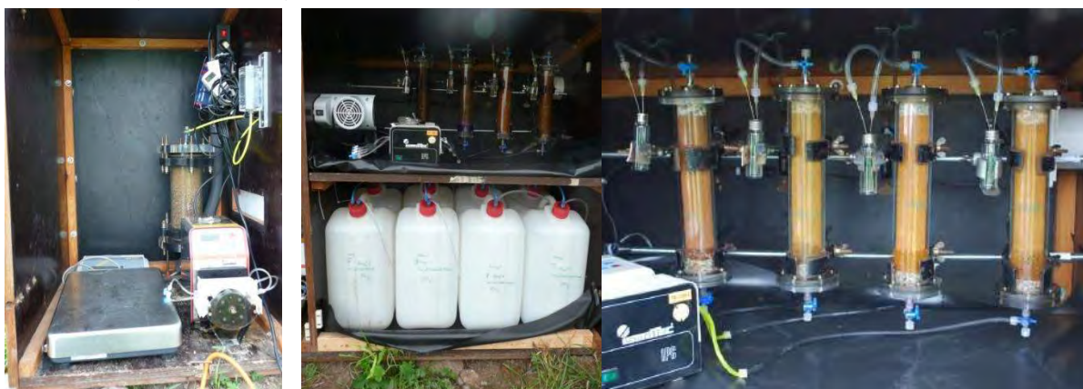
Figure 4 Field site column test design with a prefilter (sand column) and an admission pressure pump (left), the column test plant with effluent containers (middle) and the Plexiglas columns filled with adsorbents (right)
