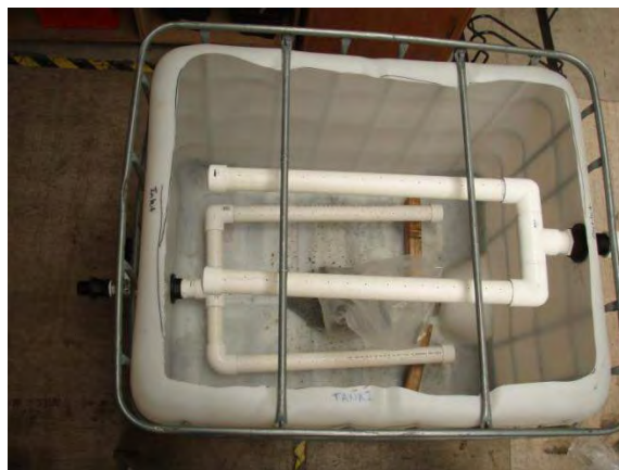
Figure 1 Adsorption chamber prior to being filled with treatment medium
