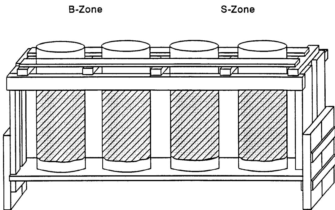
Fig. 4      Experimental arrangement of leaching columns.
