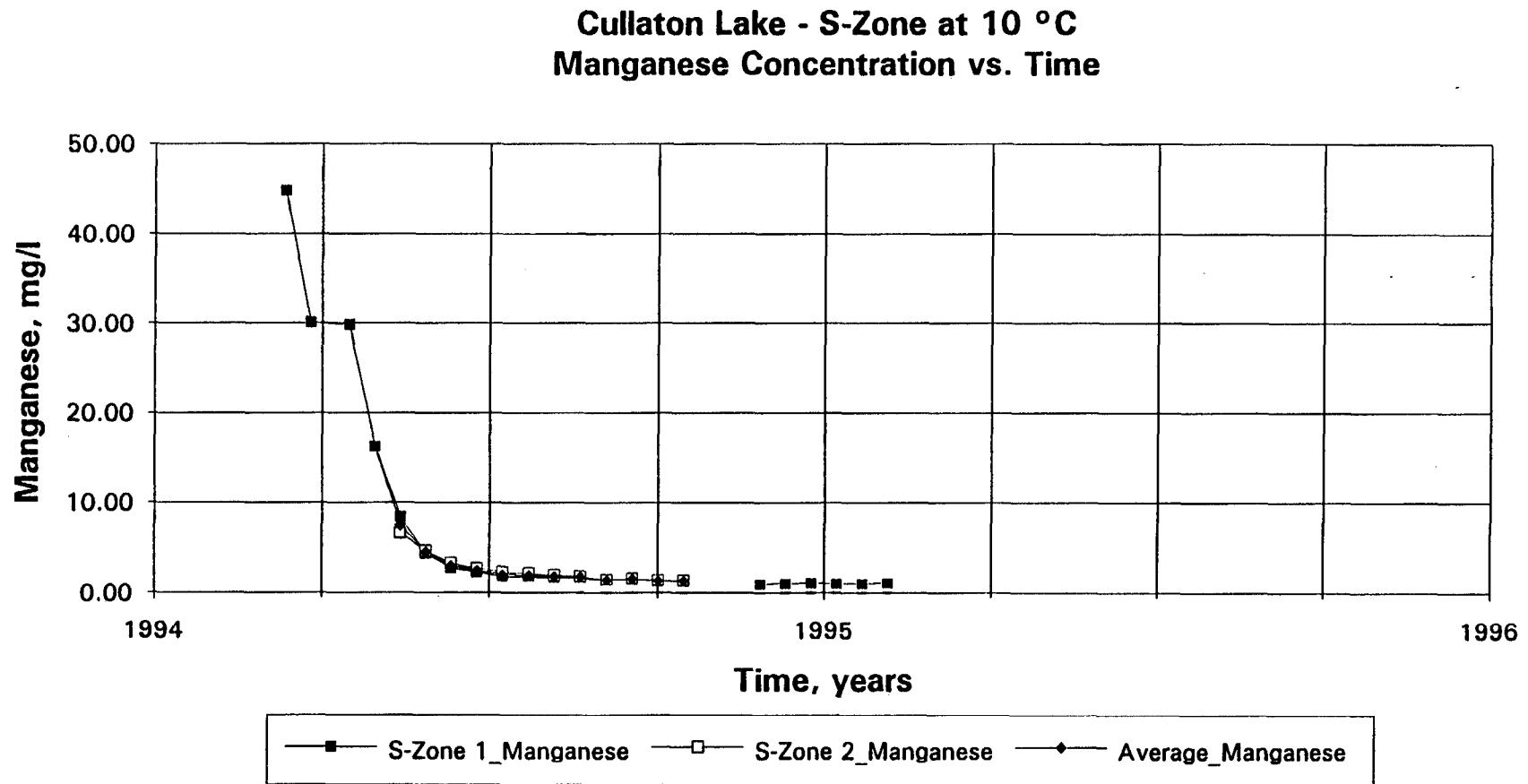
Fig. 42b S - Zone: effluent dissolved manganese concentration at 10 °C.
