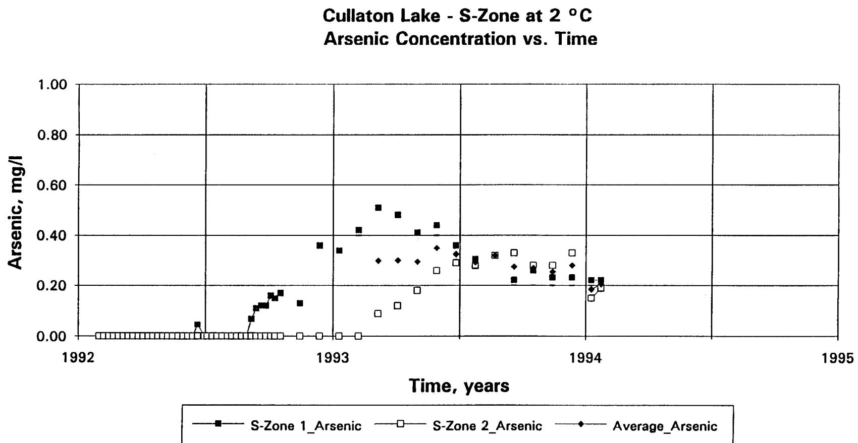
Fig. 44a S - Zone: effluent dissolved arsenic concentration at 2 °C.
