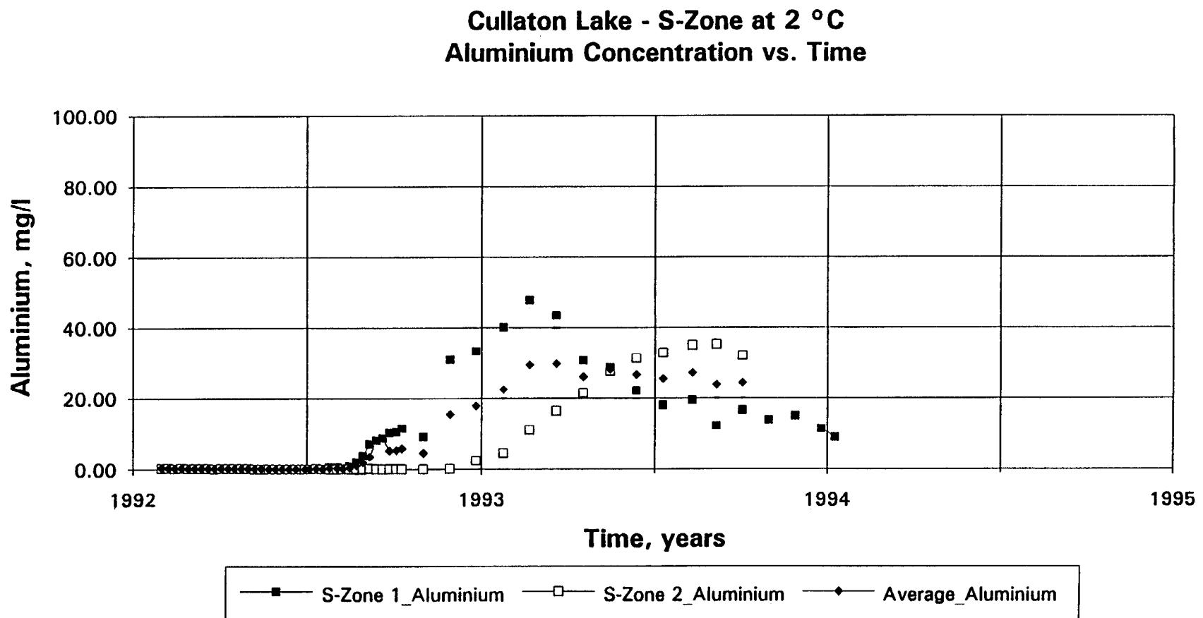
Fig. 41a S - Zone: effluent dissolved aluminium concentration at 2 °C.
