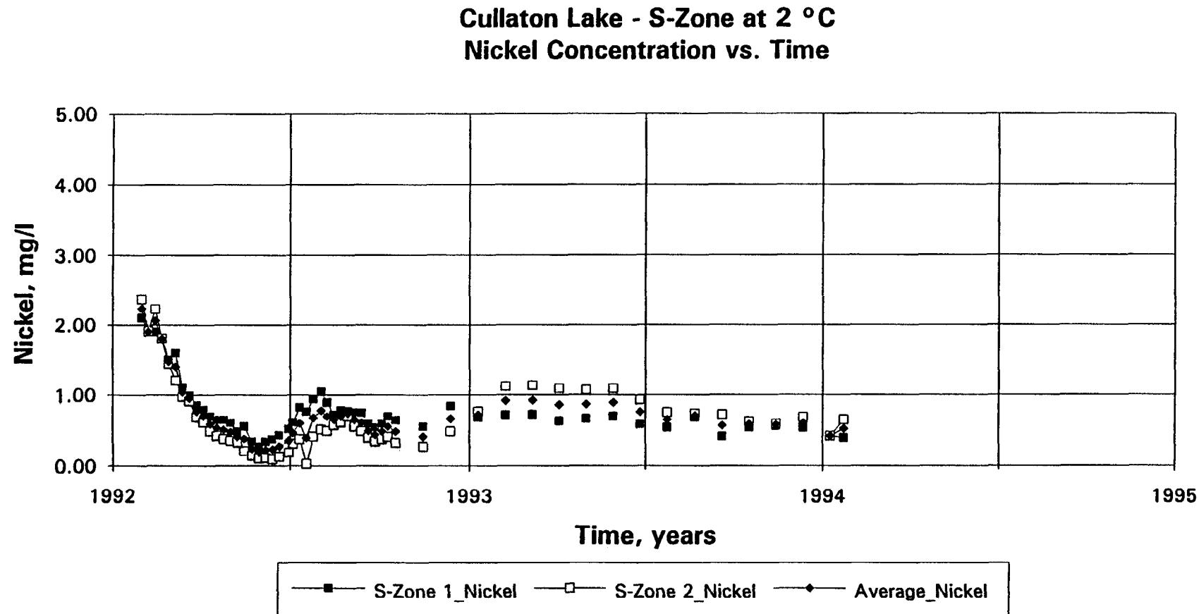
Fig. 48a S - Zone: effluent dissolved nickel concentration at 2 °C.
