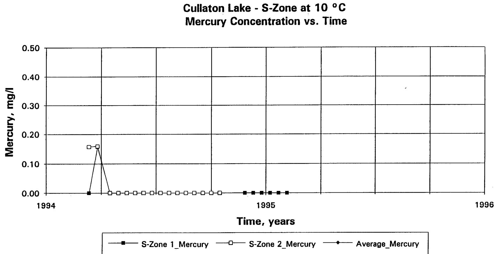
Fig. 47b S - Zone: effluent dissolved mercury concentration at 10 °C.
