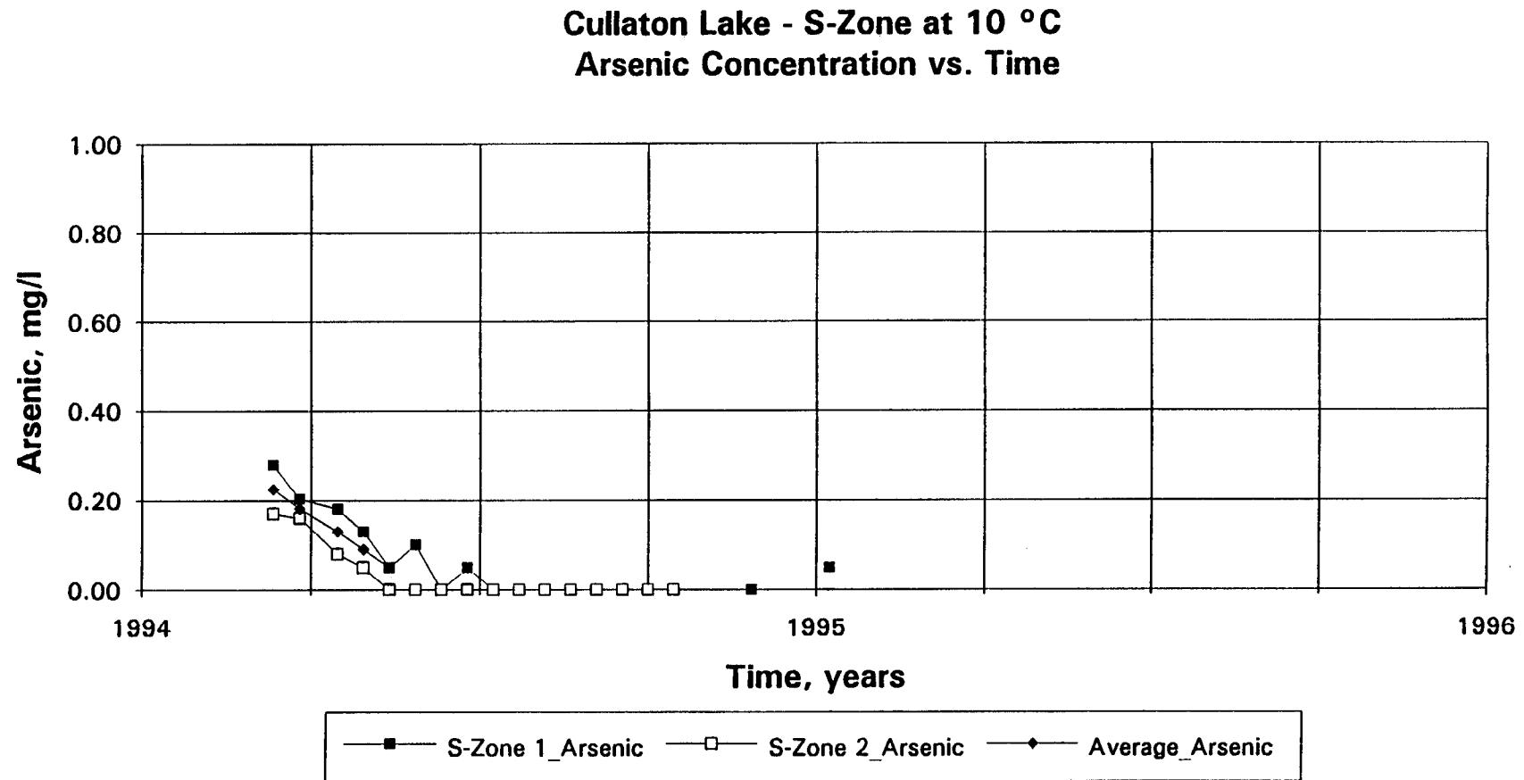
Fig. 44b S - Zone: effluent dissolved arsenic concentration at 10 °C.
