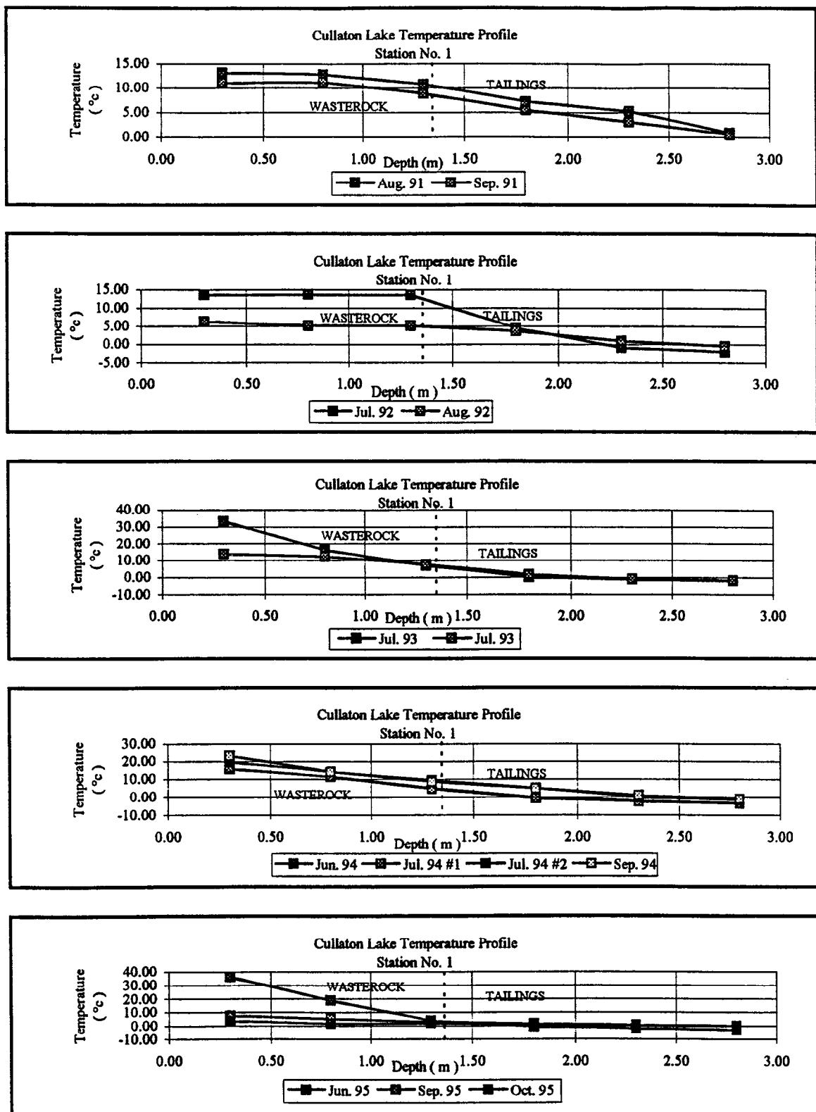
Fig. 53 Temperature profiles in wasterock and tailings at the Cullaton Lake site, Station 1.
