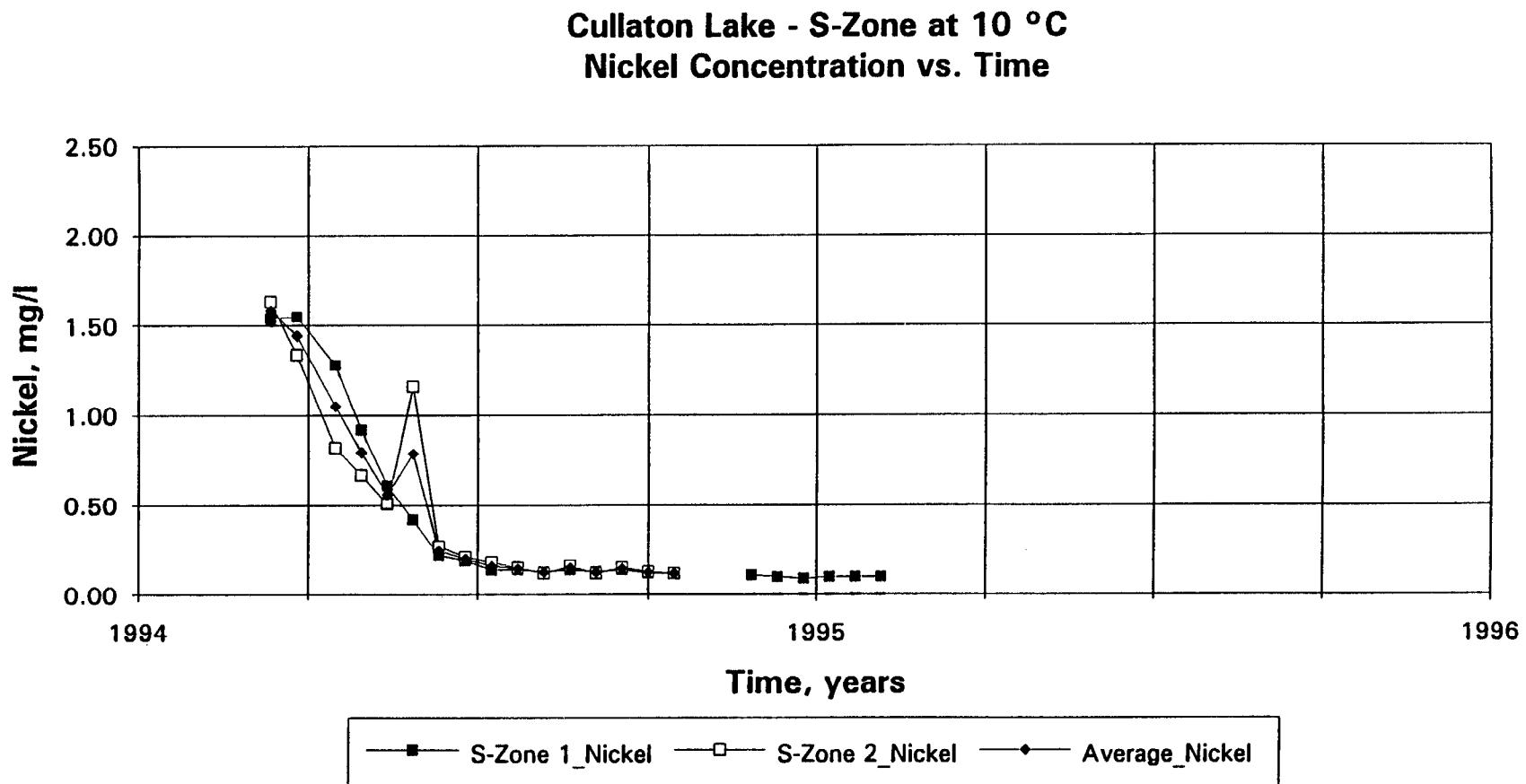
Fig. 48b S - Zone: effluent dissolved nickel concentration at 10 °C.
