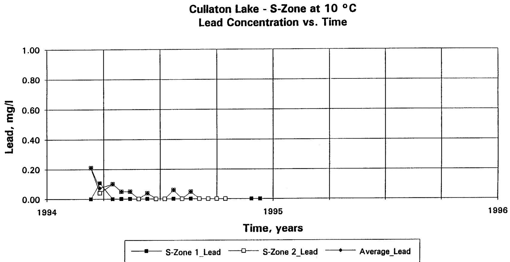
Fig. 46b S - Zone: effluent dissolved lead concentration at 10 °C.
