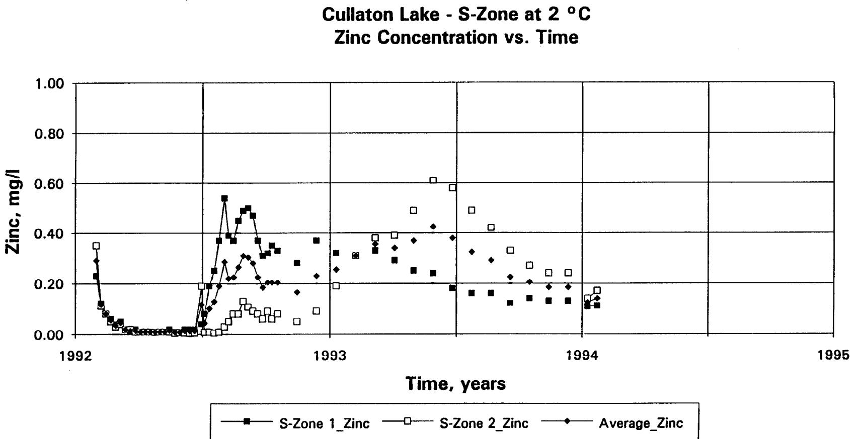
Fig. 50a S - Zone: effluent dissolved zinc concentration at 2 °C.
