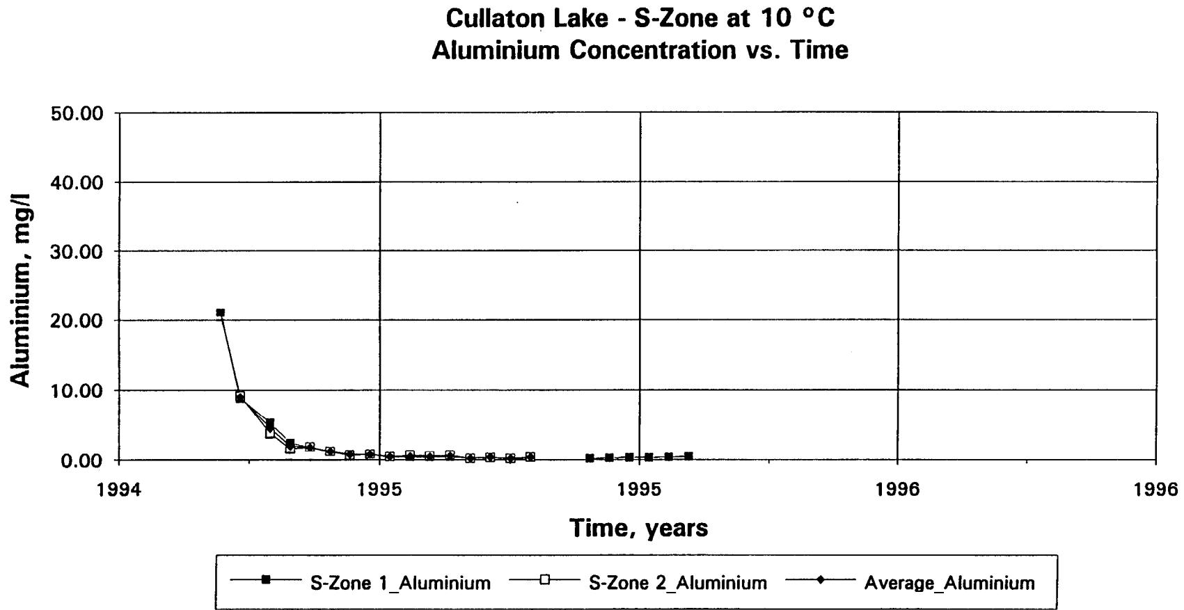
Fig. 41b S - Zone: effluent dissolved aluminium concentration at 10 °C.
