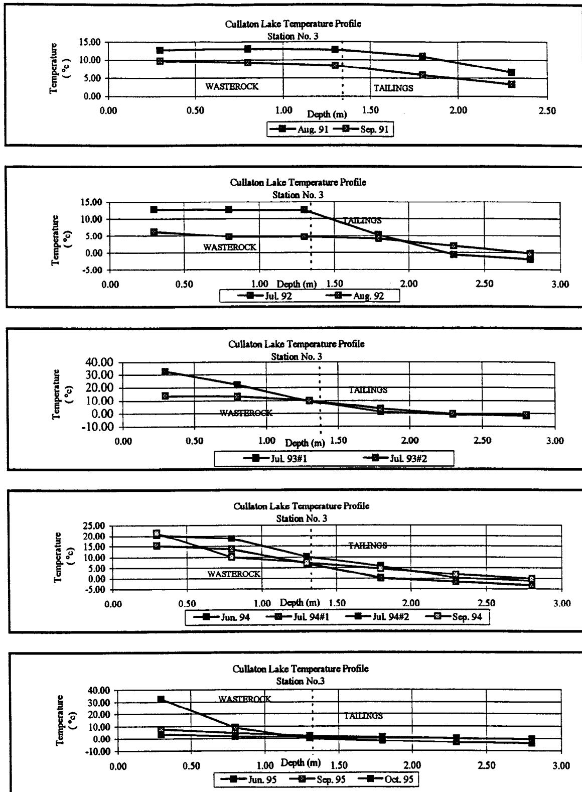
Fig. 55 Temperature profiles in wasterock and tailings at the Cullaton Lake site, Station 3.
