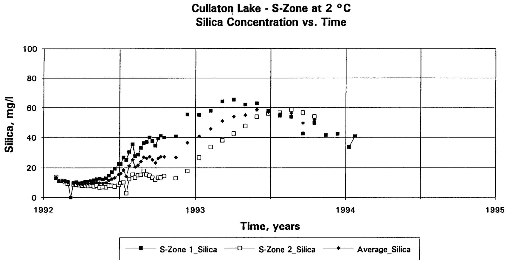
Fig. 49a S - Zone: effluent dissolved silica concentration at 2 °C.
