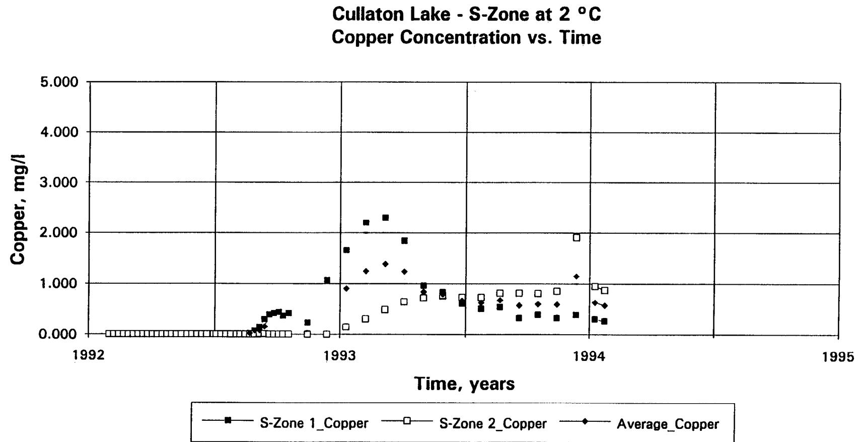
Fig. 45a S - Zone: effluent dissolved copper concentration at 2 °C.
