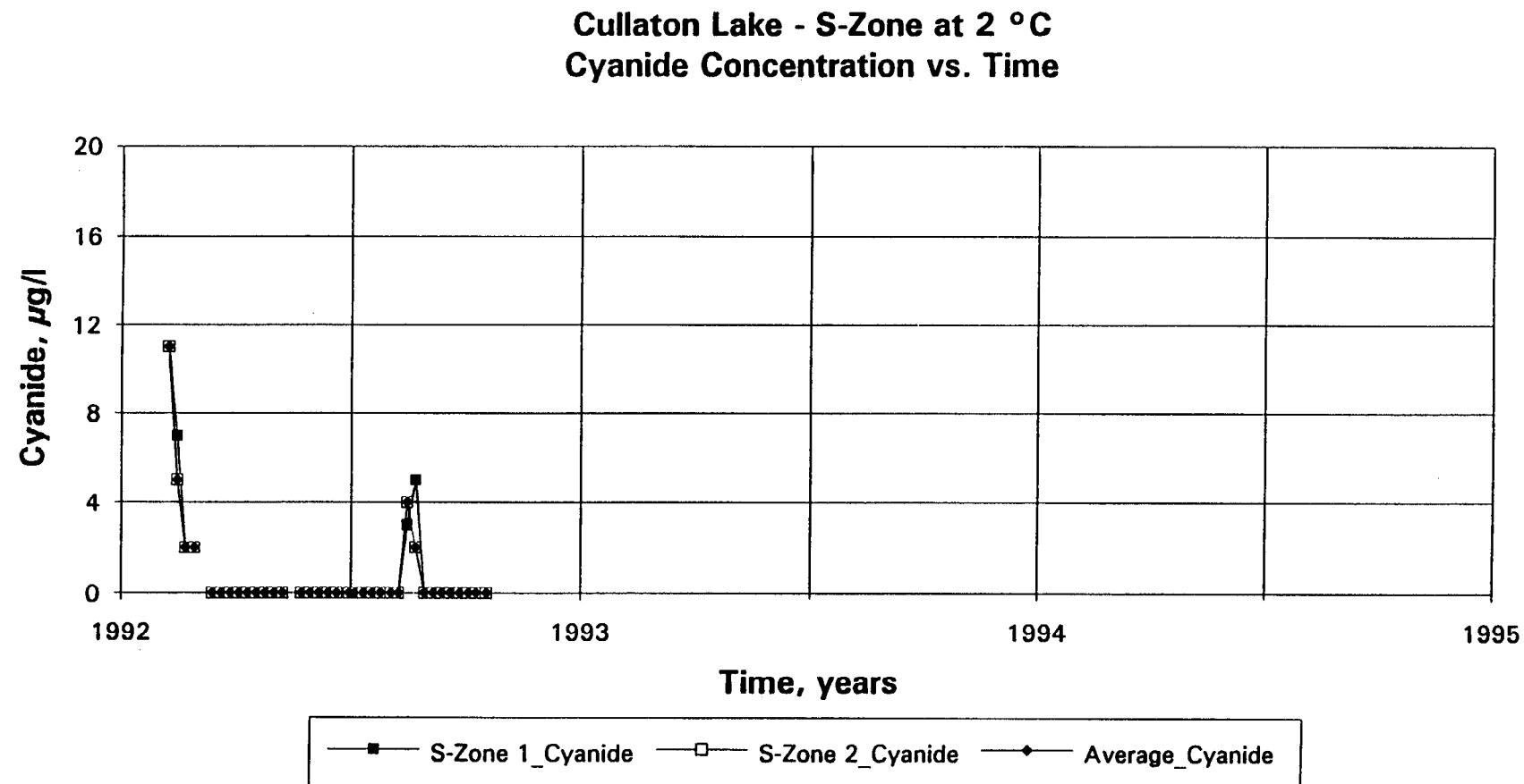
Fig. 51. S - Zone: effluent dissolved total cyanide concentration at 2 °C.
