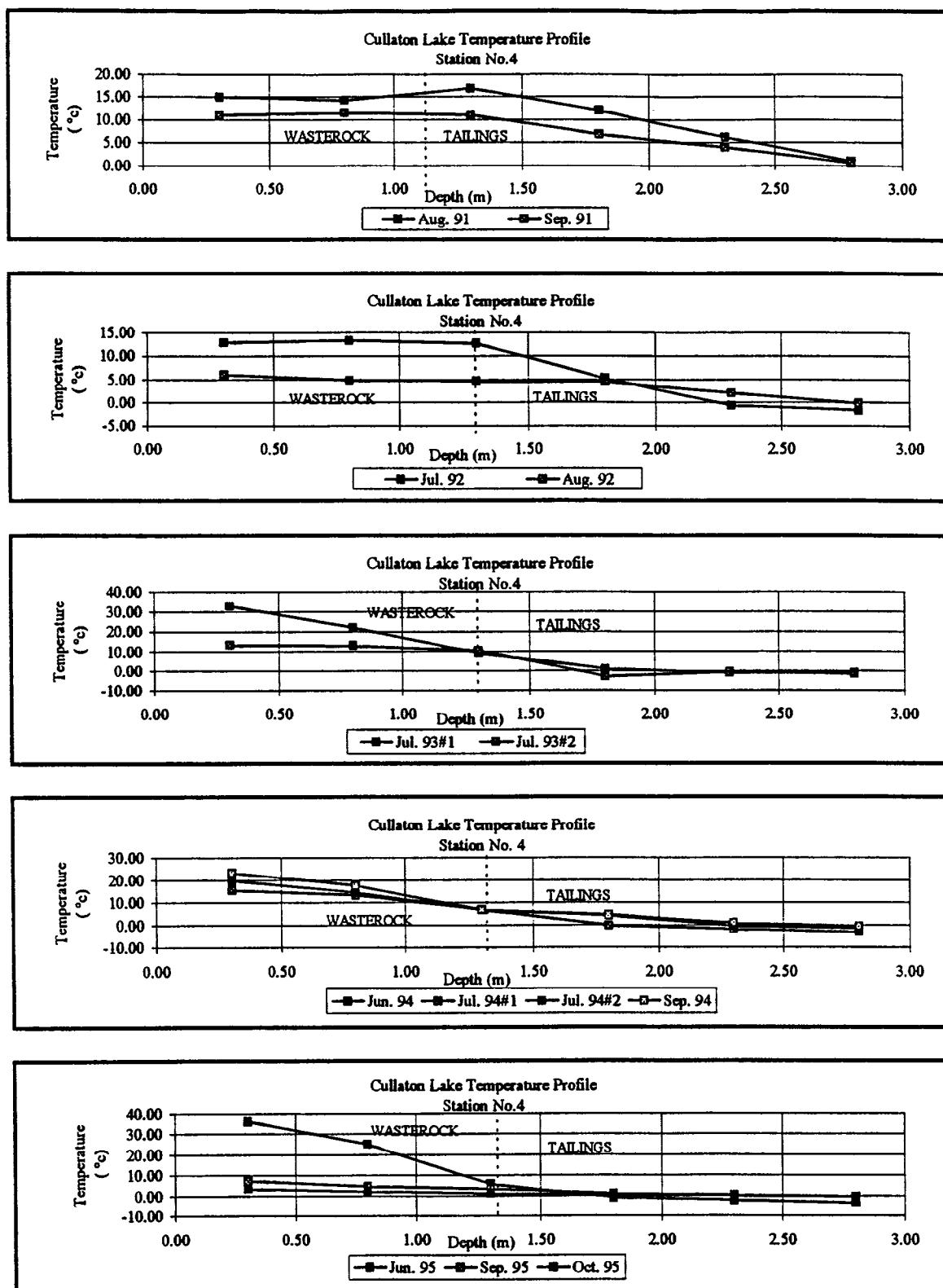
Fig. 56 Temperature profiles in wasterock and tailings at the Cullaton Lake site, Station 4.
