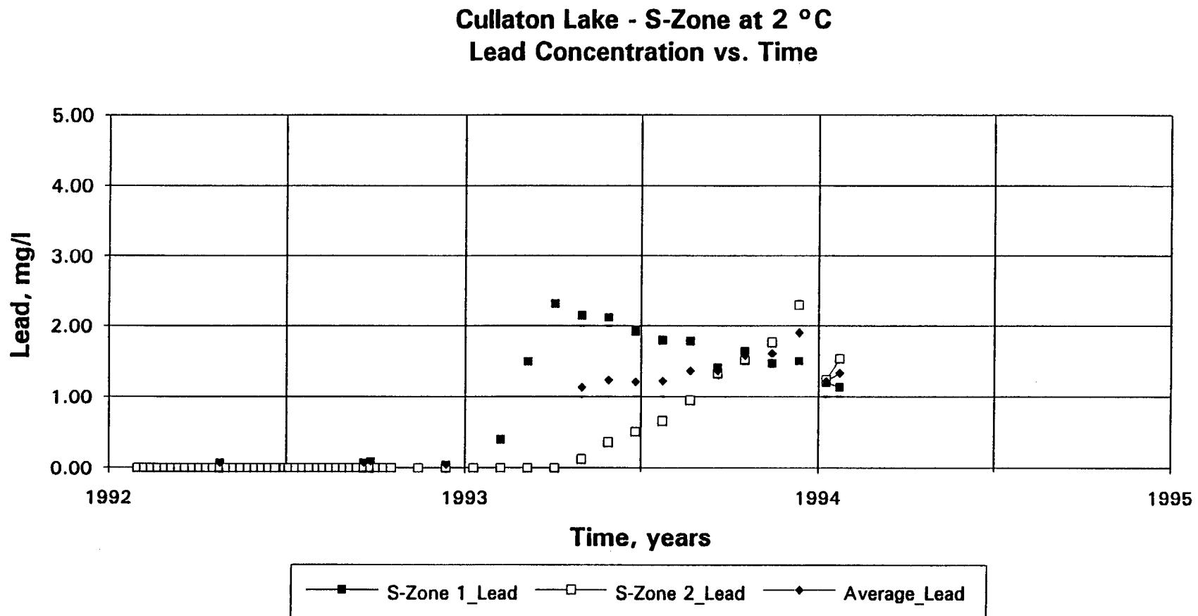
Fig. 46a S - Zone: effluent dissolved lead concentration at 2 °C.
