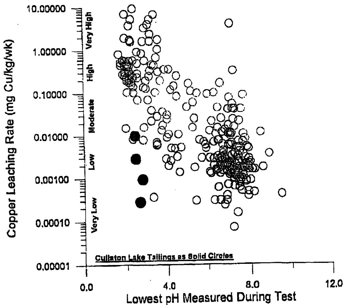
Fig. 58 International Kinetic Database: - rate of copper leaching.
