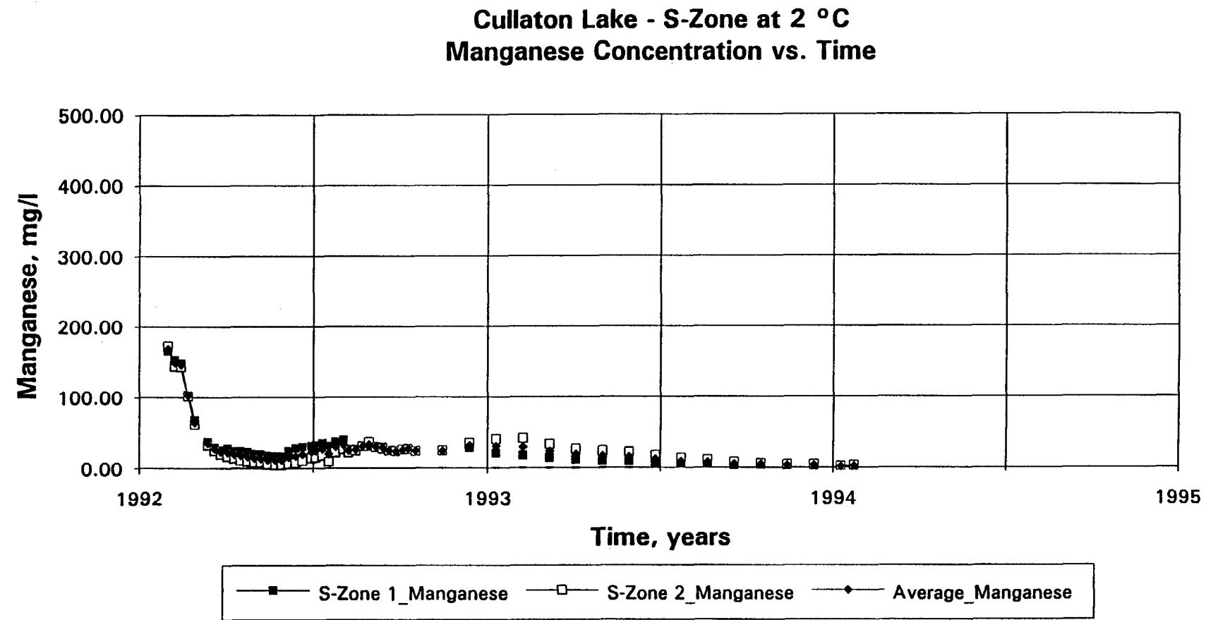
Fig. 42a S - Zone: effluent dissolved manganese concentration at 2 °C.
