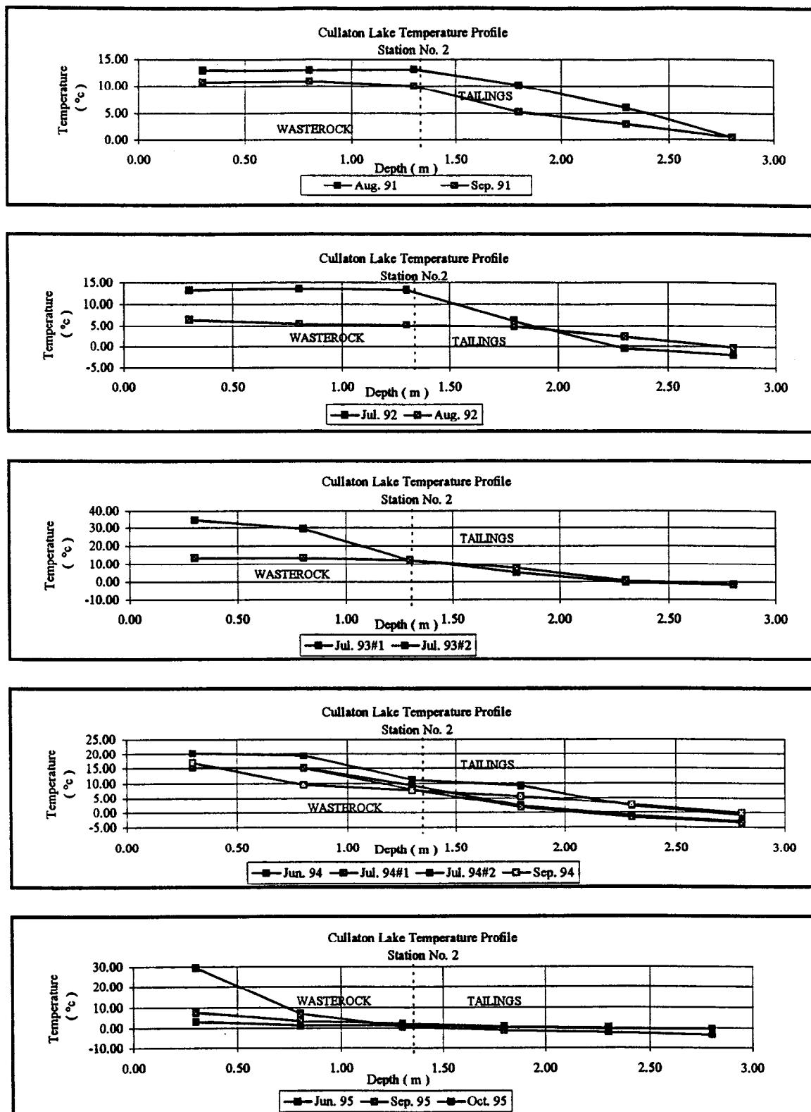
Fig. 54    Temperature profiles in wasterock and tailings at the Cullaton Lake site, Station 2.
