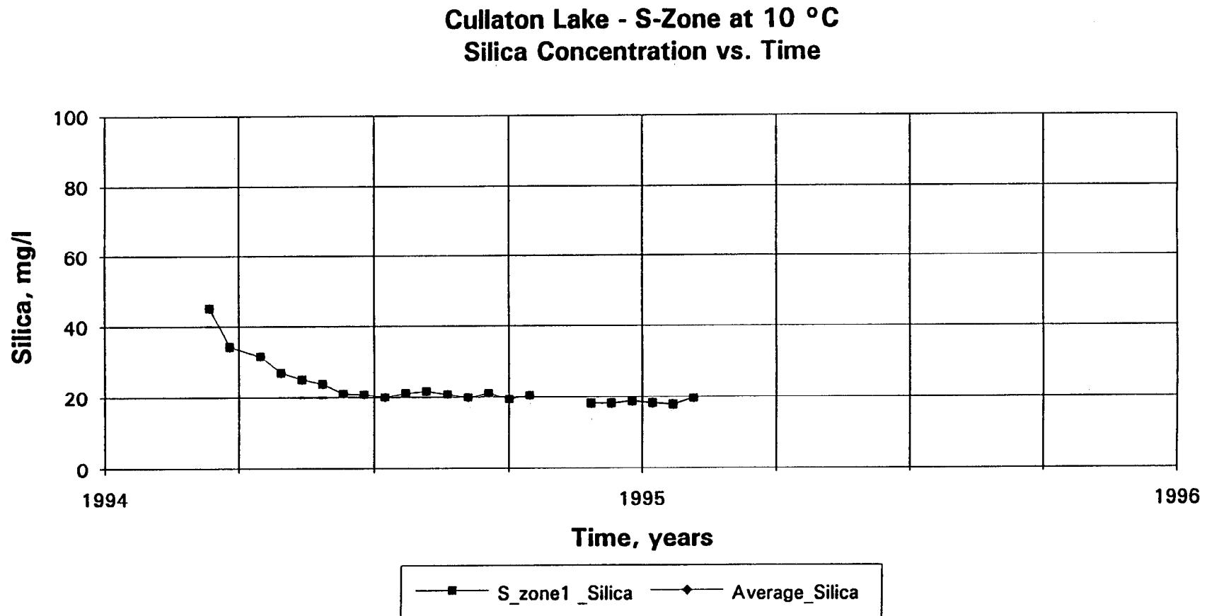
Fig. 49b S - Zone: effluent dissolved silica concentration at 10 °C.
