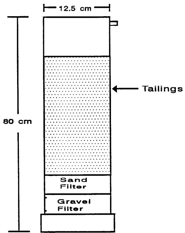
**Fig. 3** Vertical section of a leaching column.
