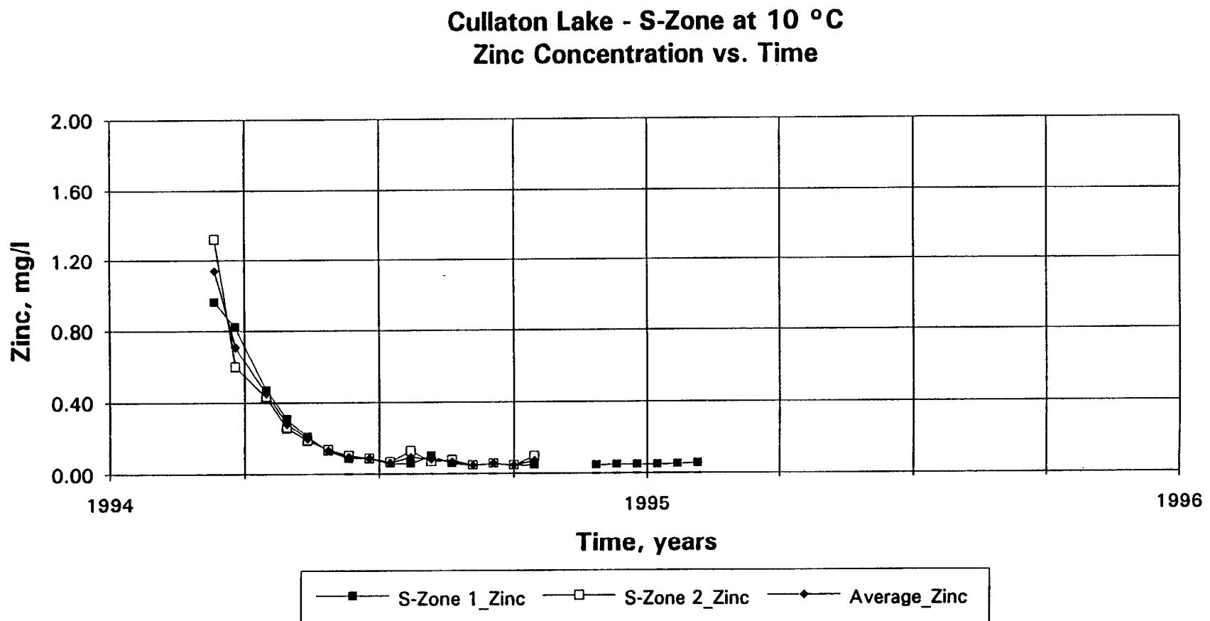
Fig. 50b S - Zone: effluent dissolved zinc concentration at 10 °C.
