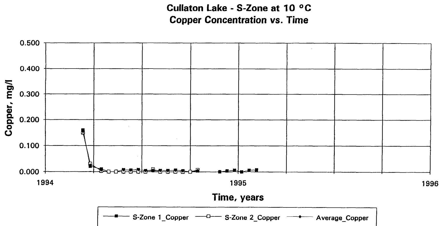
Fig. 45b S - Zone: effluent dissolved copper concentration at 10 °C.
