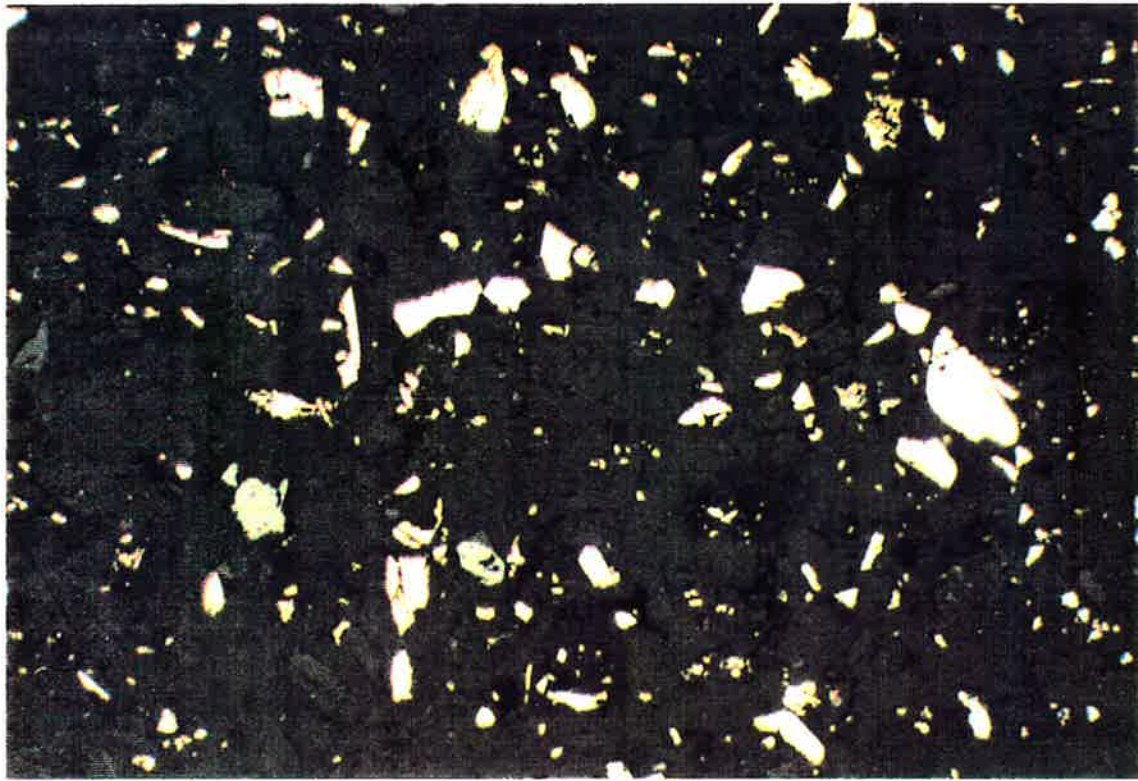
Plate 3-3: Photomicrograph of Station 1 sediments (AL-1) using reflective light (Scale 1 cm = 42 microns). Fresh pyrite (light cream colour) and gangue are found. Field included two sphalerite grains (grey) and occasional small brown grains of pyrrhotite. Note smaller particle size than in tailings.
