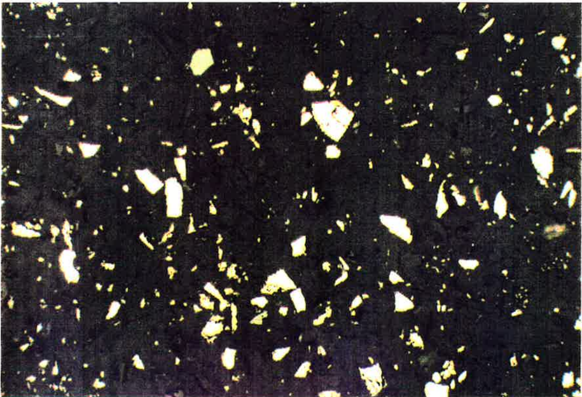
Plate 3-4: Photomicrograph of Station 2 sediments (AL-2) using reflective light (Scale 1 cm = 42 microns). Fresh pyrite (light cream colour) and pyrrhotite (slightly browner grains) are seen. Note higher abundance of gangue than Station 1.
