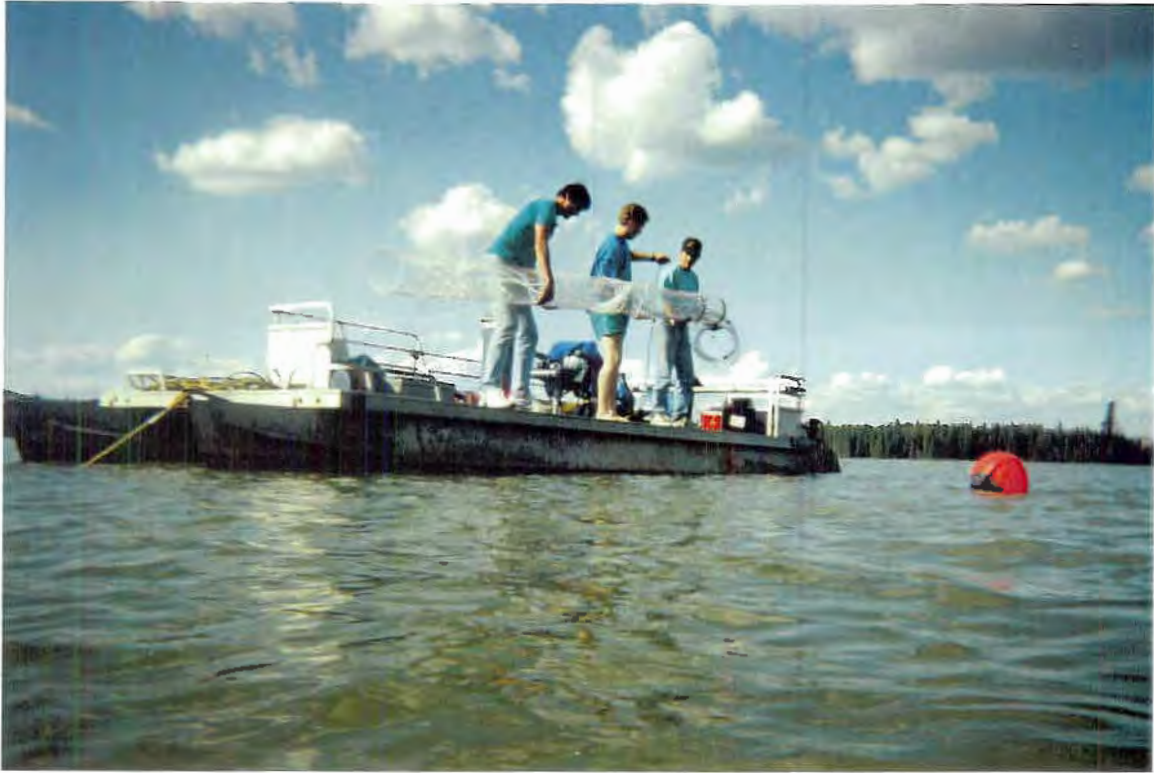
Plate 2-1: In situ water column sampler utilized in the Anderson Lake Surveys.
