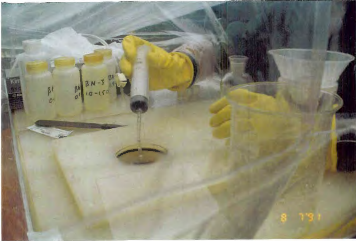
Plate 2-10: Commencement of core sectioning in N_2 - filled glove bag of the extrusion table.
