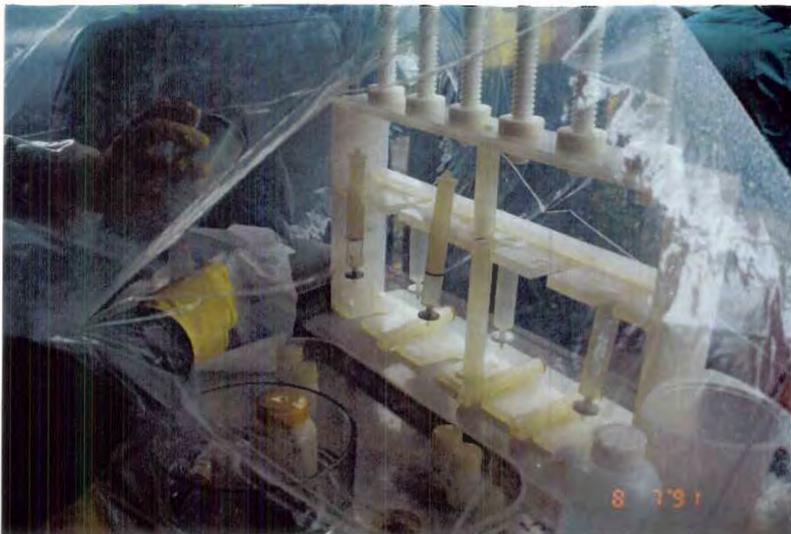
Plate 2-11: Porewater filtration in secondary N_2 - filled glove bag.
