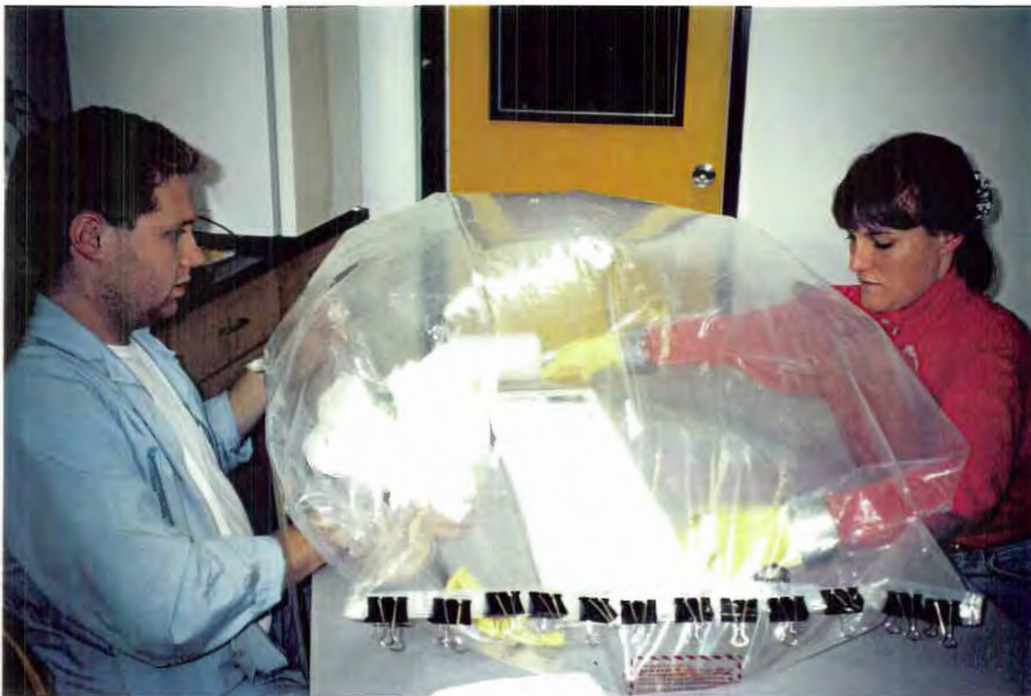
Plate 2-14: Subsampling of Rescan peeper in a N_2 - filled glove bag.
