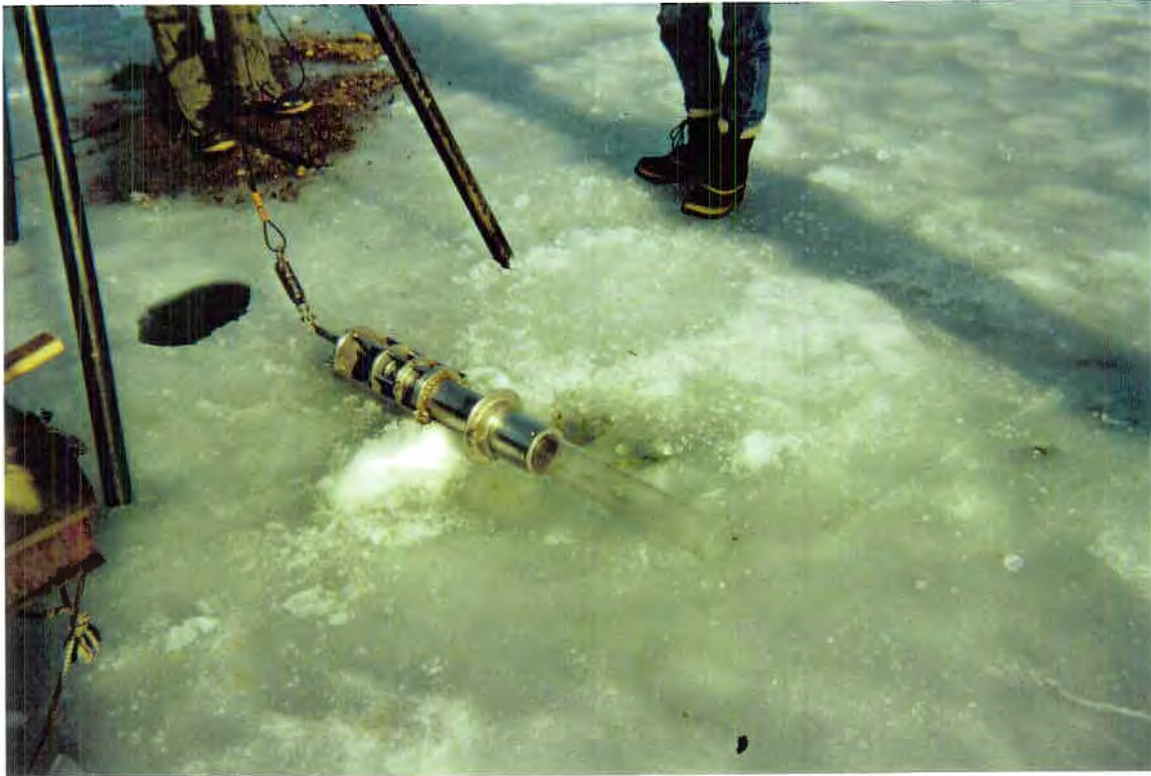
Plate 2-7: Pedersen corer, and tripod prior to coring at Station A.
