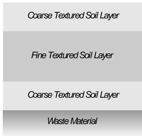
Figure 2.6 Multi-layer cover system over waste material.
