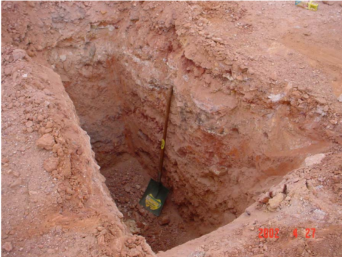
Figure 3.1 A 2.0 m test pit excavated in waste rock material.
