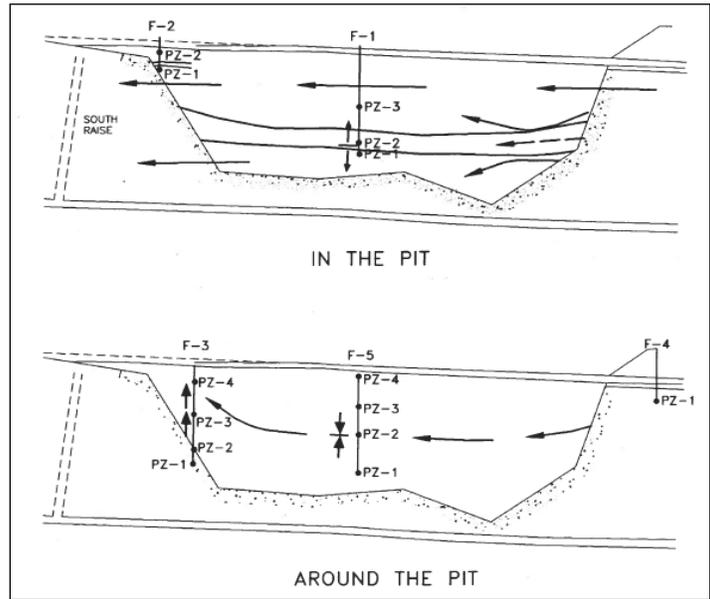
**Figure 3-10 Schematic Section of Solbec Open Pit Showing Average Calcium Concentration (mg/L) in Groundwater (1993) [7]**
