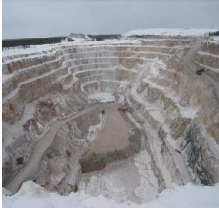
**Figure 10-19 Water-covered Waste Rock in the Sue C Pit [22]**
