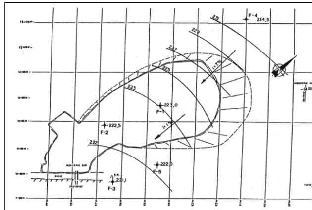
**Figure 3-9 Groundwater Flows Within and Around the Solbec Pit (1994) [7]**
