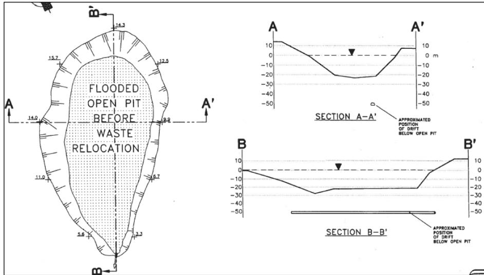
Figure 3-4 Longitudinal Section of the Solbec Pit (1987) [7]
