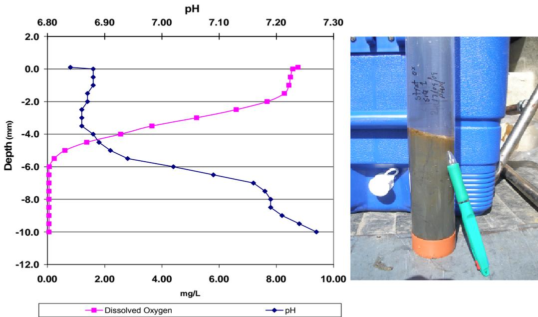
**Figure 11** Micro-pH and dissolved oxygen profiles measured in the sediment core from Sampling Site 1 at the Strathcona Mine.
