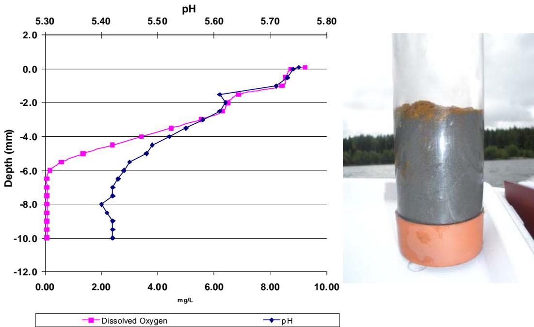
**Figure 10** Micro-pH and dissolved oxygen profiles measured in the sediment core from Sampling Site 3 at the Louvicourt Mine.
