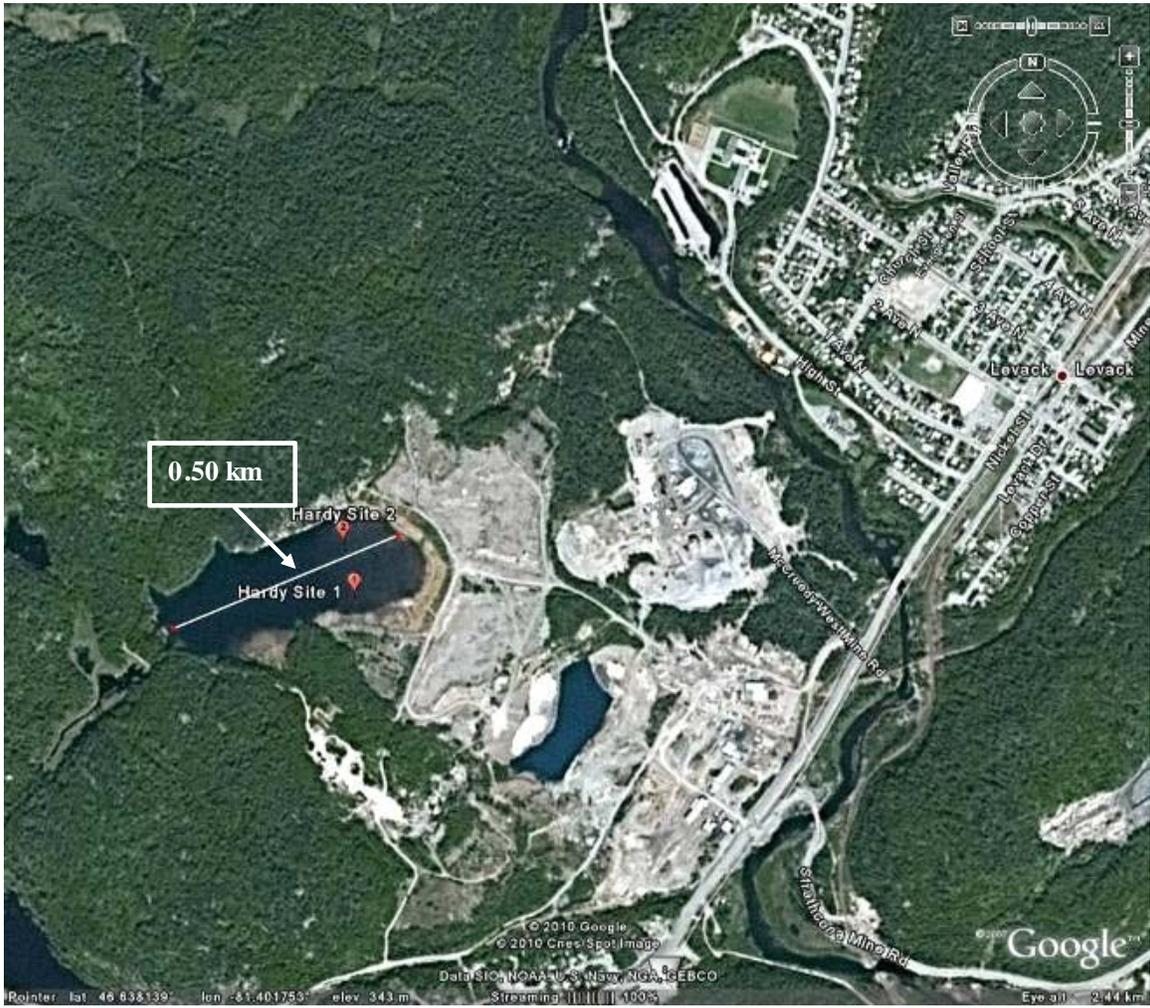
Figure A-5 Size of the tailings pond and sampling sites at the Hardy Mine.
