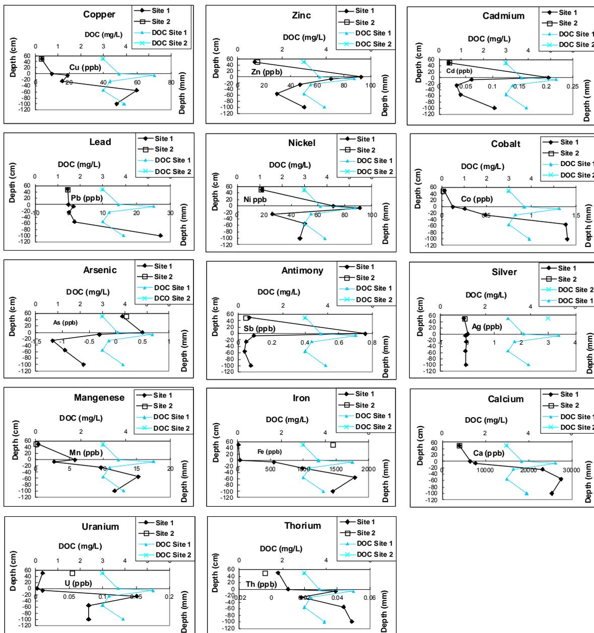
**Figure 6** Variation of water chemistry with depth at the Hardy Mine tailings pond. (Note that water depth is in cm (+) above and in mm (-) below the interface (0); insufficient porewater was extracted from Site 2 sediment for metals analysis)
