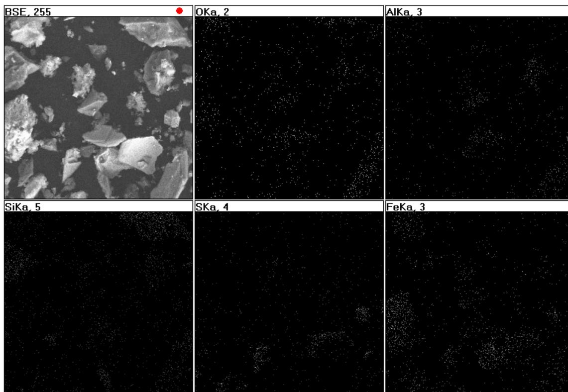
**Figure 4** A backscattered electron image (BSE, top left; 1000X magnification) of a subsample of the Louvicourt tailings collected at the water/sediment interface and the corresponding X-Ray maps for O, Al, Si, S and Fe. Bright clusters associated with ferrihydrite (e.g. upper left corner, lower left and near middle of BSE where the X-Rays maps show no S associated with Fe) are biofilm aggregates. The white, platy grain at the lower right corner where Fe and S are found together is pyrite.
