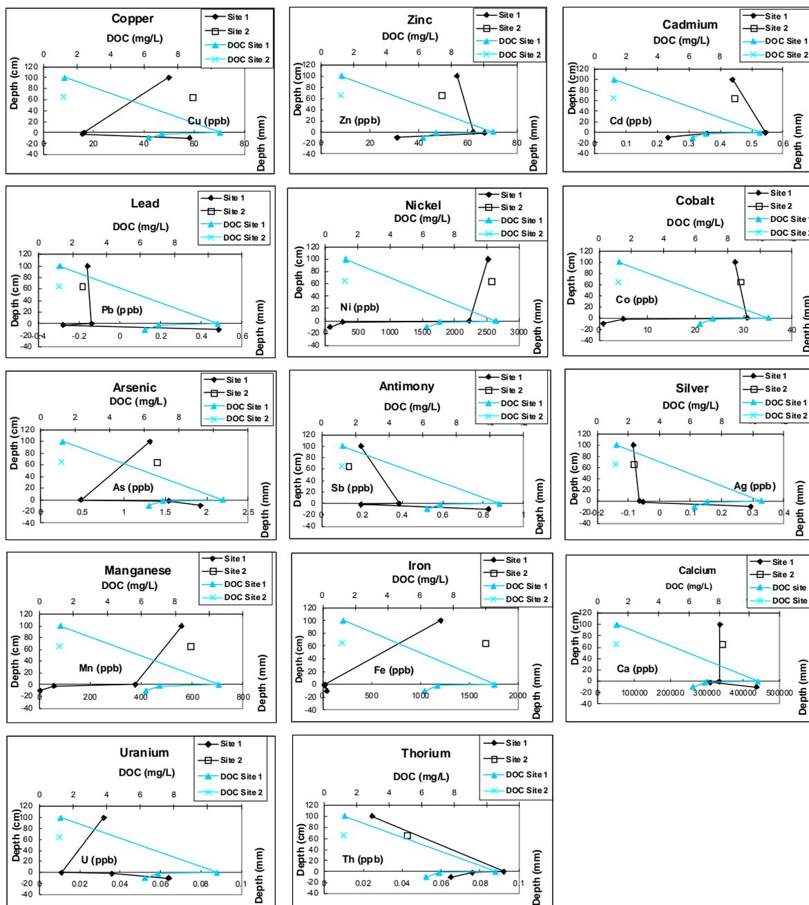
**Figure 7** Variation of water chemistry with depth at Moose Lake, Onaping Operation. (Note that water depth is in cm (+) above and in mm (-) below the interface (0); insufficient porewater was extracted from Site 2 sediment for metals analysis)
