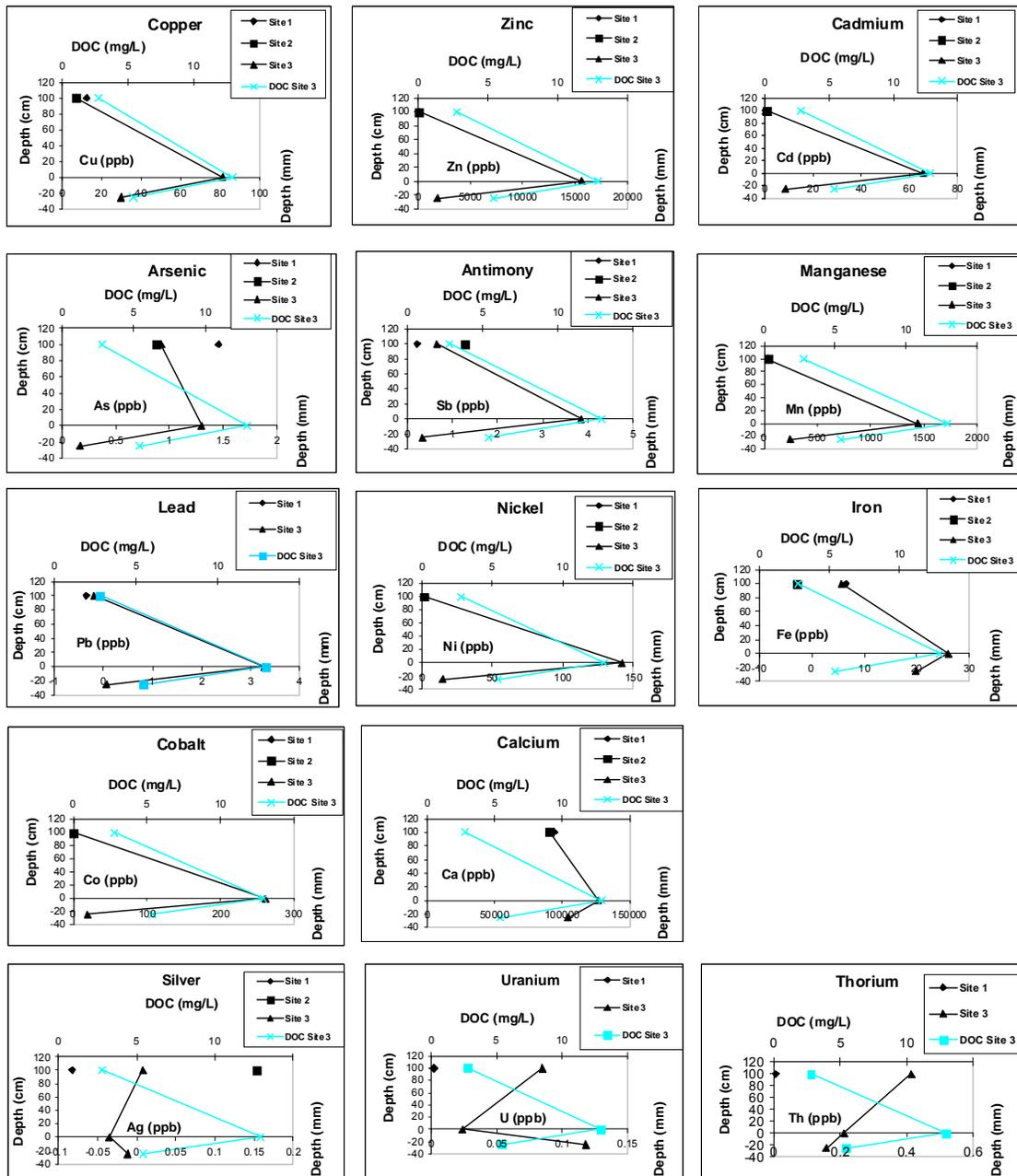
**Figure 3** Variation of water chemistry with depth at the Louvicourt tailings pond. (Note that water depth is in cm (+) above the water/tailings interface (0) and in mm (-) below the interface.)
