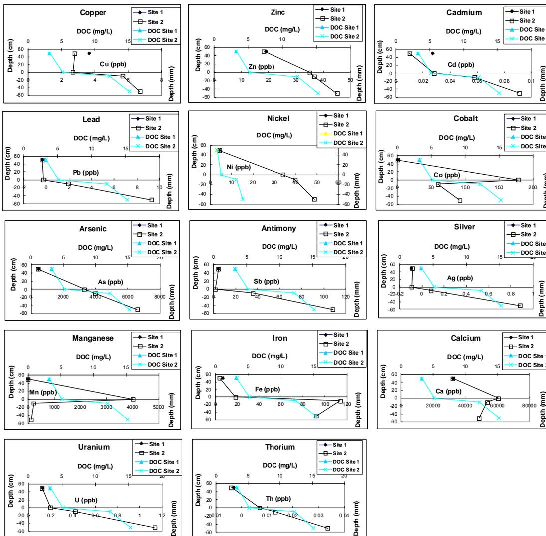
**Figure 5** Variation of water chemistry with depth at the Nova Scotia tailings pond. (Note that water depth is in cm (+) above the tailings/water interface (0) and in mm (-) below the interface; insufficient porewater was extracted from the sediment core collected from Site 1 for metals analysis.)
