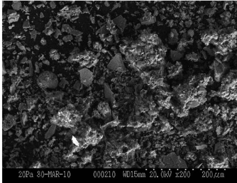
**Figure 8** Backscatter electron image of a tailings subsample from the Denison TMA1 at 200X magnification. The bright grain at the lower left is monazite (a rare earth phosphate). The scattered light gray patches covering some larger grains are iron monosulfide and microbes. The gray minerals in the matrix are largely quartz with minor amounts of K-feldspar, mica, calcite and pyrite.
