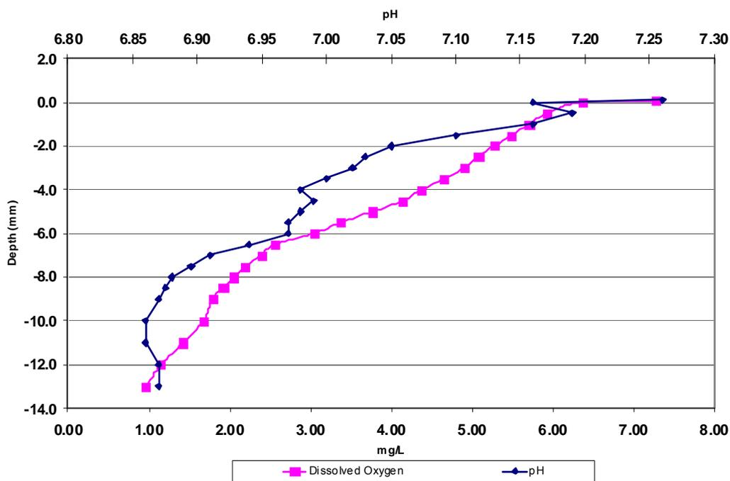
**Figure 12** Micro-pH and dissolved oxygen profiles measured in the sediment core from Sampling Site 3 at the Hardy Mine.
