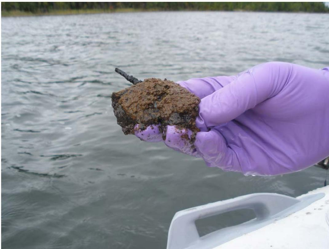
**Figure 2** Loose patches of biofilm found on submerged tailings at the Louvicourt tailings impoundment.
