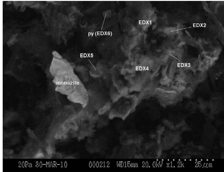
**Figure 9** Enlarged (1200X) BSE image of the SW quadrant of Figure 8. *In-situ* spot EDX analyses at locations EDX 1-6 confirm that they are composed of iron monosulphide associated with silica and carbon.
