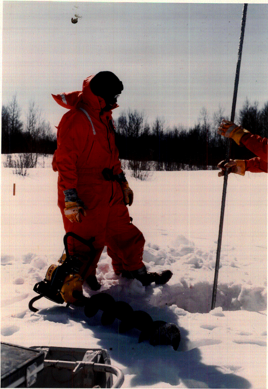
Figure 3: Winter sludge sampling using a hand corer.
