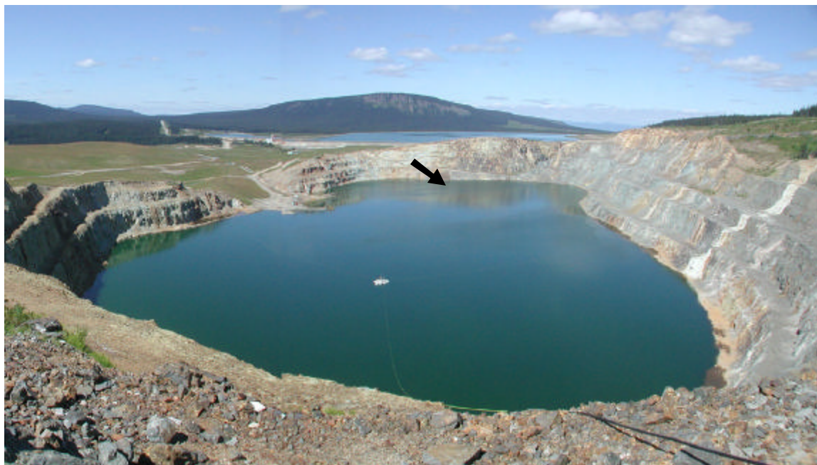
Figure 14 - Main Zone Pit at Equity Silver Mine. Arrow points to sludge addition location.
