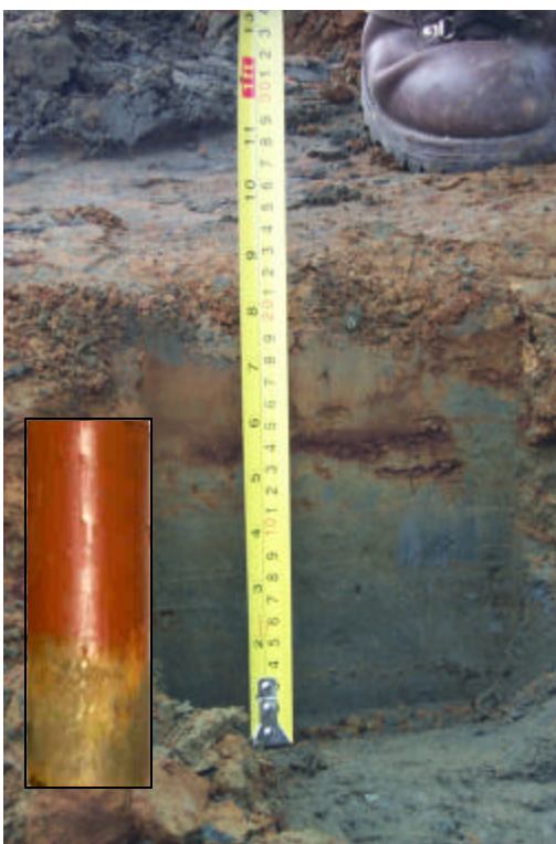
Figure 9 - Field example of sludge layered over tailings. Inset shows a core of sludge over tailings disposal scenario.
