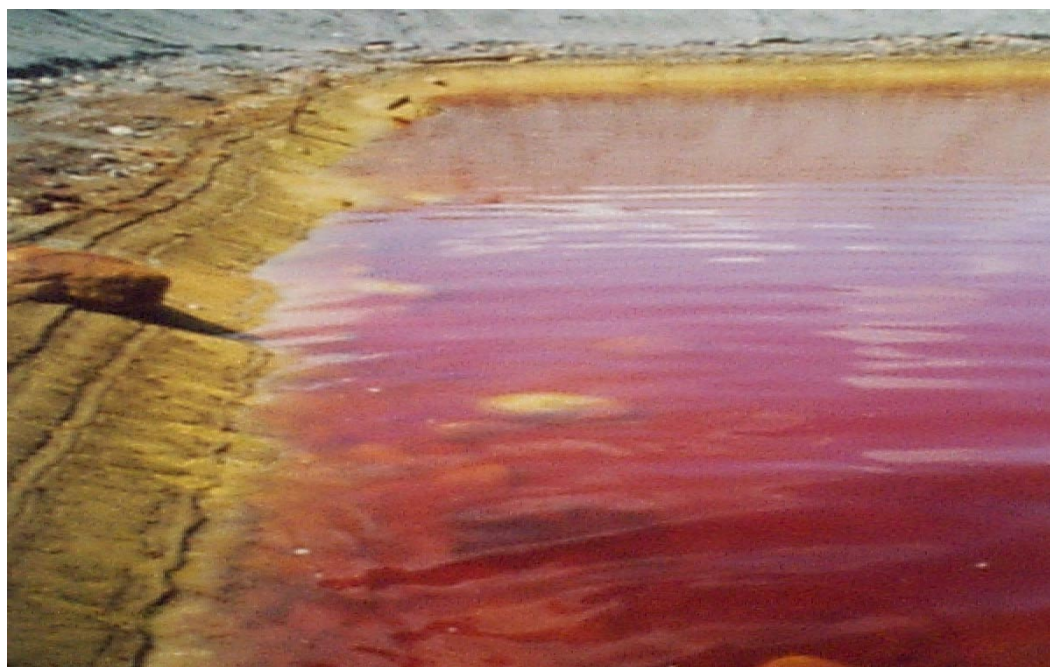
Figure 3-7: Photograph of test cell showing hydrous ferric oxide precipitate
