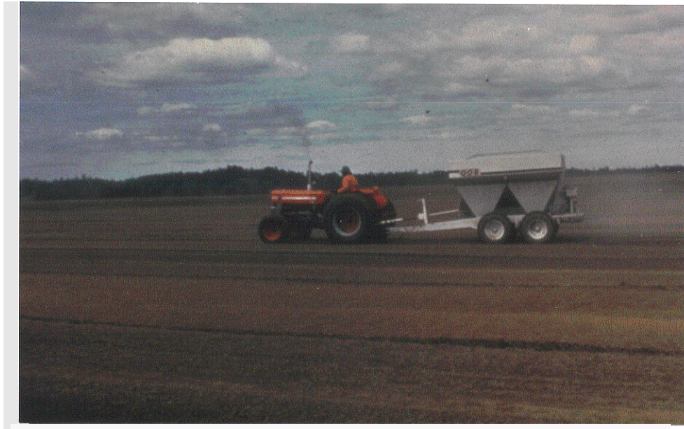
Photo 7 Cyclone Type Spreader
