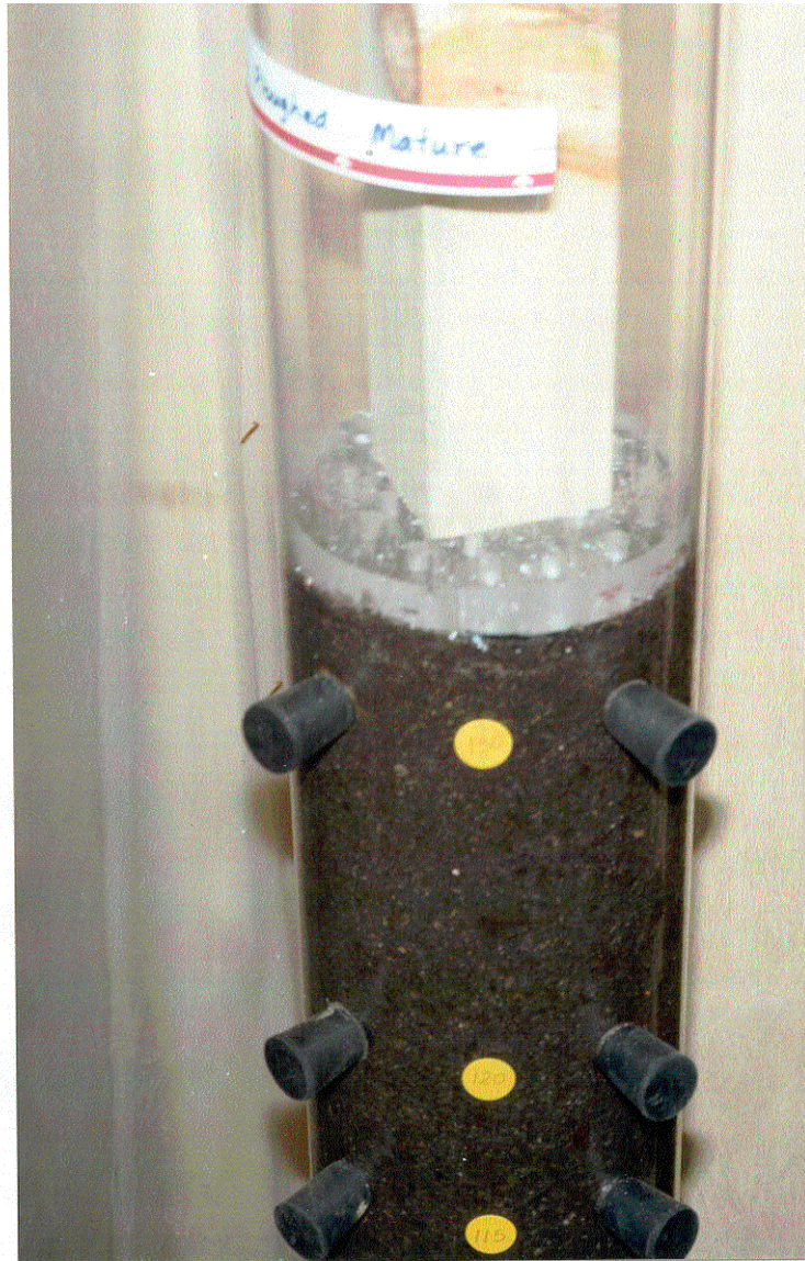
Photo 2. Close view of a plexiglass disk attached to a pine post inside a leaching column. With the addition of weights at the top of the post this became a piston for compacting the compost layer.
