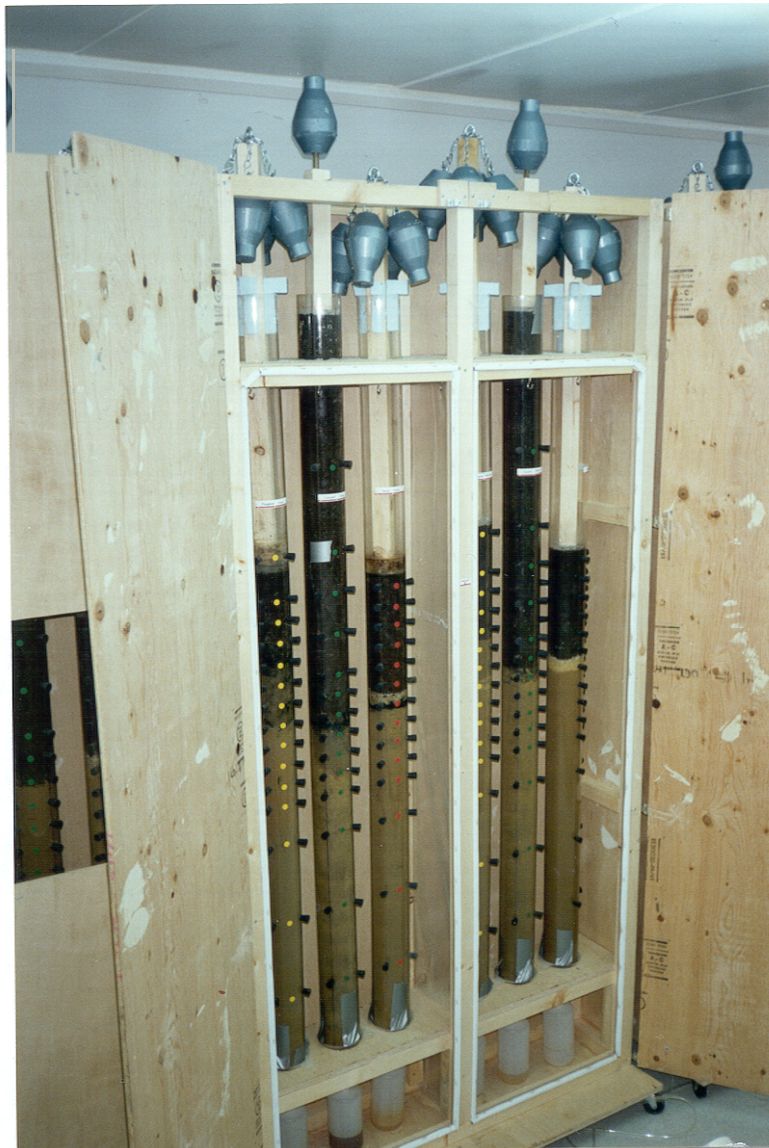
Photo 1. Nitrogen atmosphere cabinet containing six leaching columns - one replicate of the three cover layer models for the two grades of compost.
