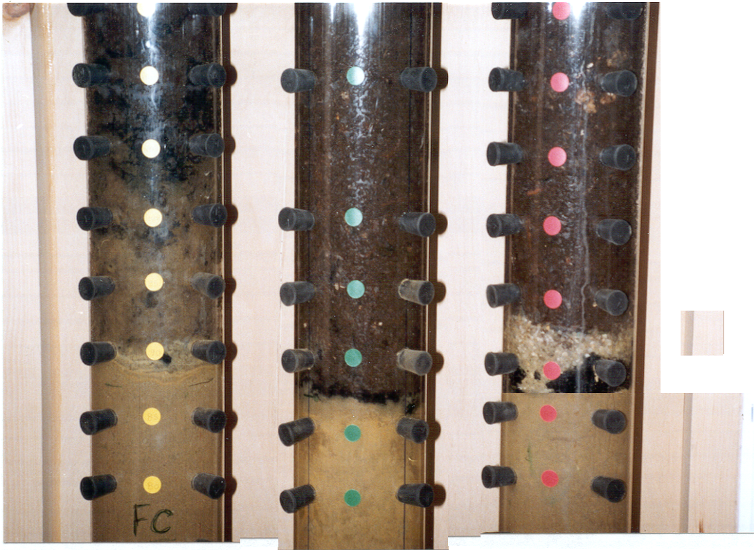
Photo 4. Three leaching columns containing fresh compost. The Ploughed model is on the left, Compost model is in the middle, and the Sand model is on the right. Note the formation of black iron sulphide precipitate near the compost-tailing interface.
