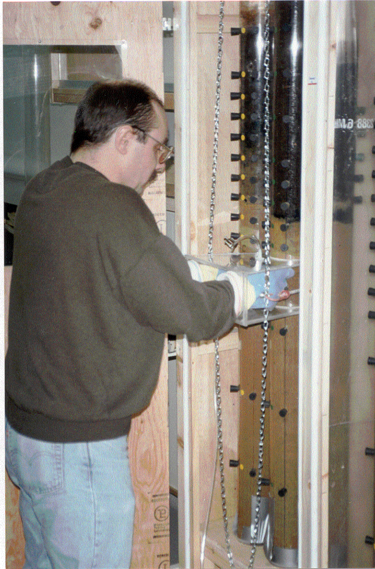
Photo 7. Sampling glove box in use on a leaching column. Notice the two chains and elastic cord supporting the box while the experimenter takes the samples. The nitrogen line is visible feeding into the top of the box.
