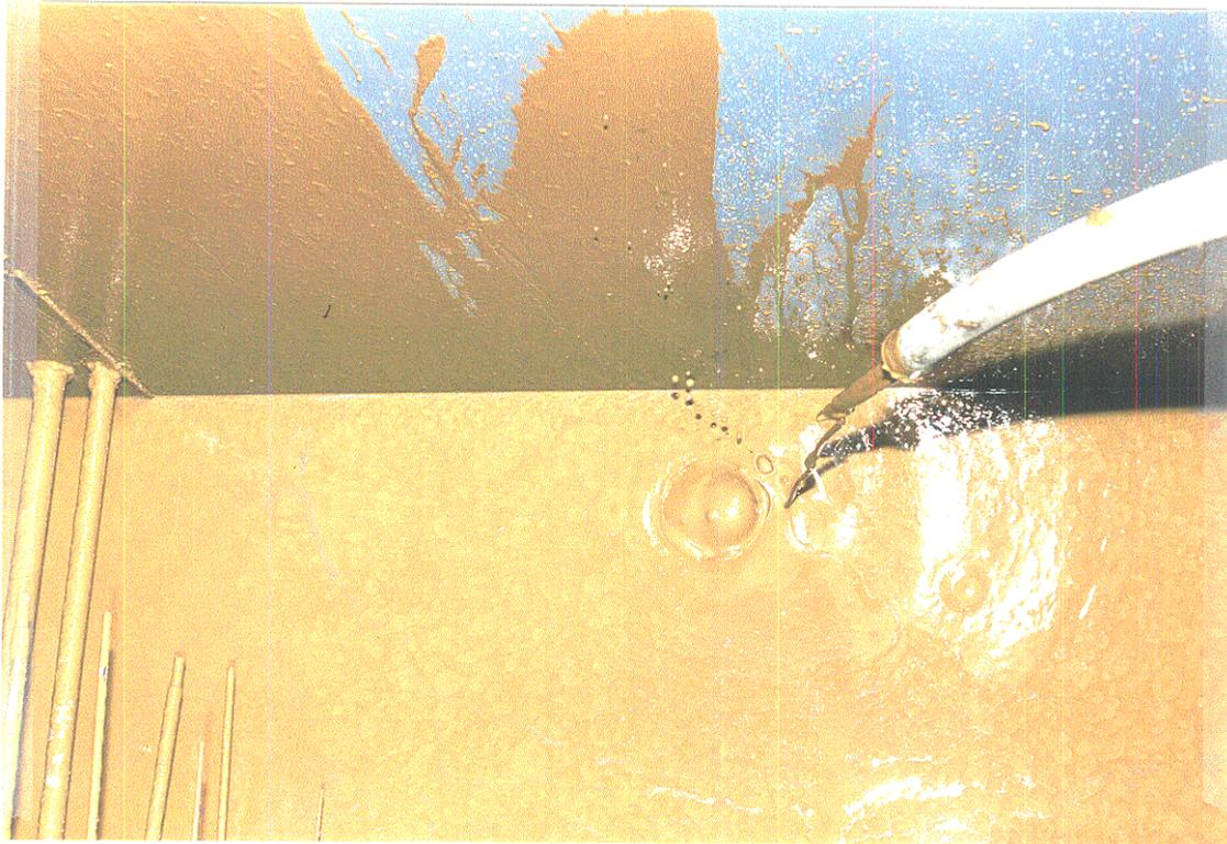
**Plate #6: Filling Pilot Cell with Tailings**
