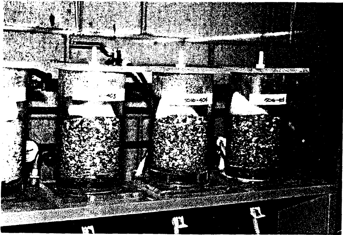
Plate 6-1: Phase I laboratory humidity cell tests. Twenty two humidity cells each contained one kilogram of rock representing the major rock types in the Sumac adit.
