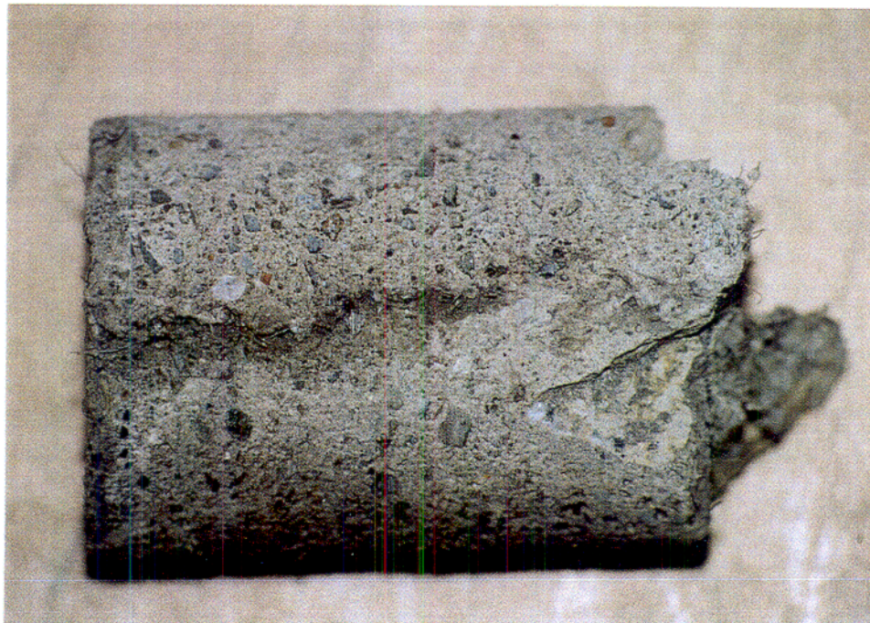
Photo 12 A core drilled in November 1992, with a crack terminated in the cover
