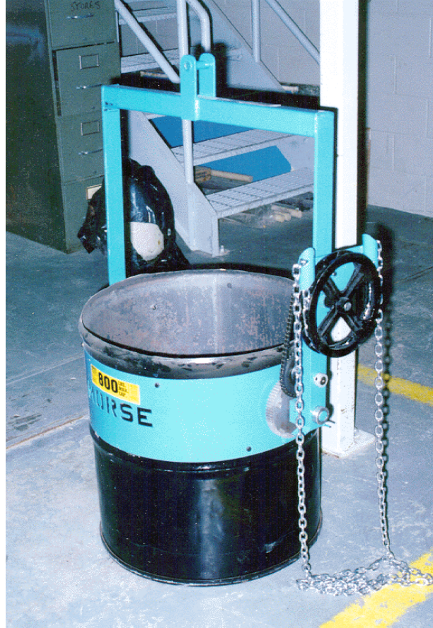
Figure 2-11 Drum Loader Used for Loading Rock into Columns
