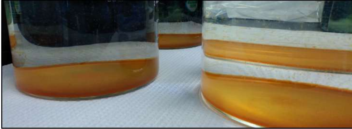
Figure 3-3: Settled Column of 20:1 Fe:As Molar Ratio Dosage After 24 Hours Settling
