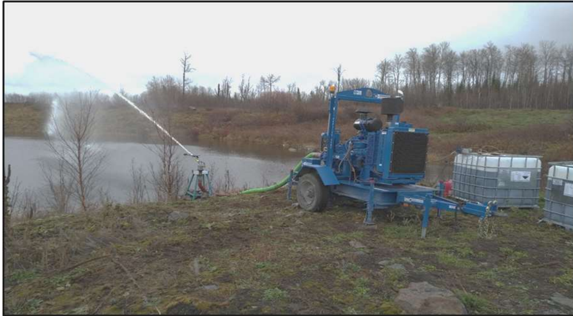
Figure 5-1: Spray Application showing Totes of Ferric Sulphate at Right, Pump and Water Cannon
