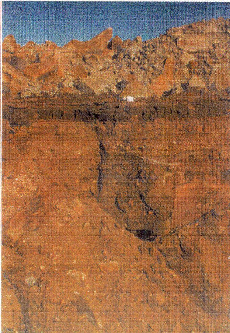
**Photos E-4. Test pit four - artificially baffled area on waste rock used to deposit / contain sludge deposited fall '93. Sludge layered 1) top 2-3" cracked 2) stratified layers 3) still moist sludge beneath upper waste rock. Looks like a "low porosity chimney" or vent which was filled with sludge.**
