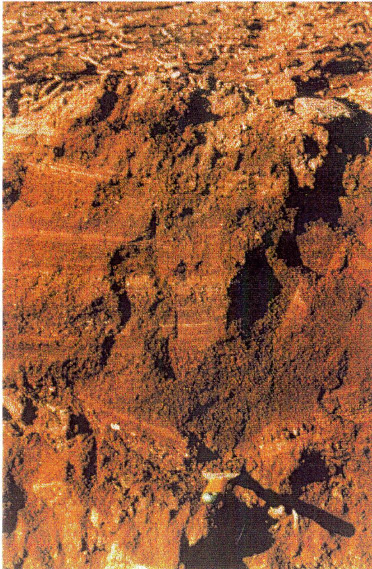
**Photos E-3. Test pit three - sludge deposited by dredging, fall '93. Sludge very powdery. Weeds with rhubarb shaped leaves / growth on surface. Sludge is stratified. Note tiny granules on figure 3 that are still undehydrated sludge at 24" below surface.**
