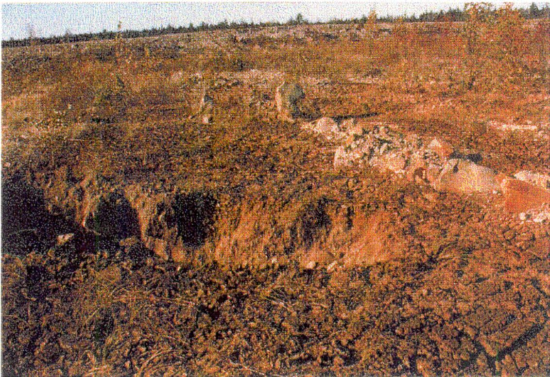
**Photo E-1. Test pit 2 sludge deposited fall '93. Area previously vegetated. Vegetation (mostly grasses and yellow birch(?)) continued to grow through sludge. Neutralization plant is at upper left (on top picture). Dried sludge layered above weathered waste rock.**
