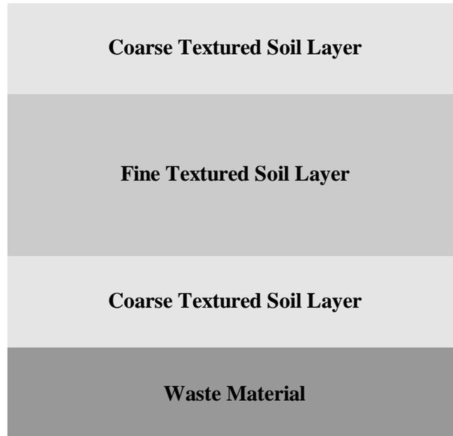
Figure 2.3 A soil-cover system over waste material (from O’Kane 1996).
