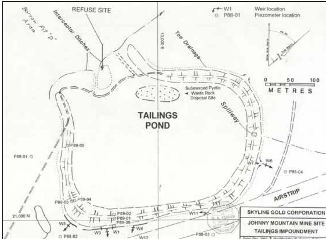
Figure 6. A Map of the Tailings Impoundment showing the Location of Waste Rock Deposition
